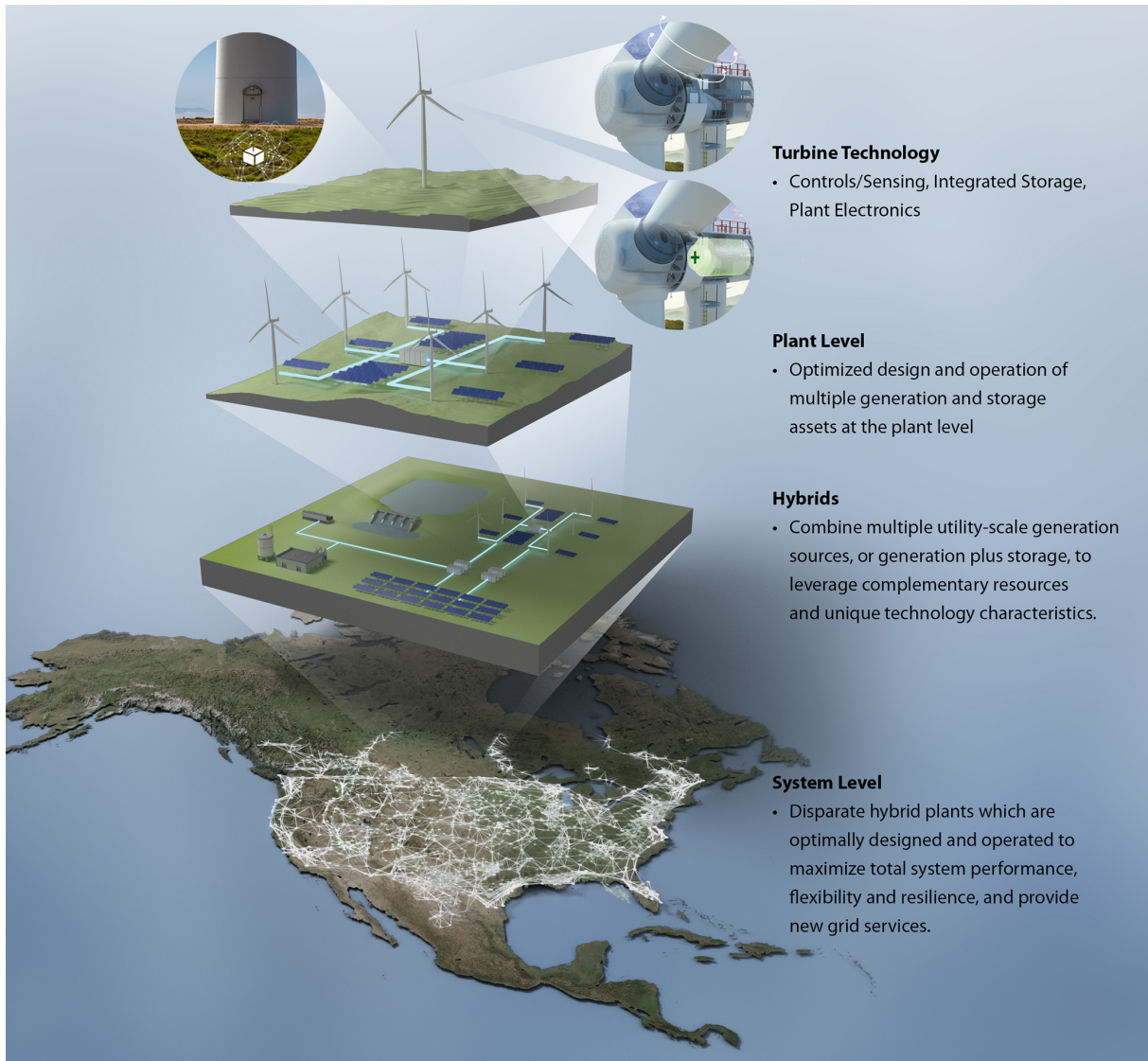
Figure 4. Wind turbine to plant to hybrid to power system level and the provision of services to meet the power system needs.
