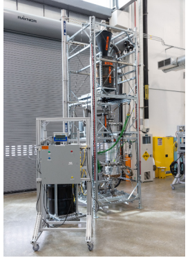
Above Left: PUMP test structure at NREL ESIF laboratory. Above Right: PUMP test structure CAD to illustrate all components including the FB HX (light blue) and particle conveying technologies used to control FB height and operating parameters: mechanical screw conveyor (red) controls FB particle outflow, L-valve (cyan) controls FB particle inflow, and pneumatic conveyor (dark blue) transports particles in return loop. Below: L-valve and screw conveyor.
