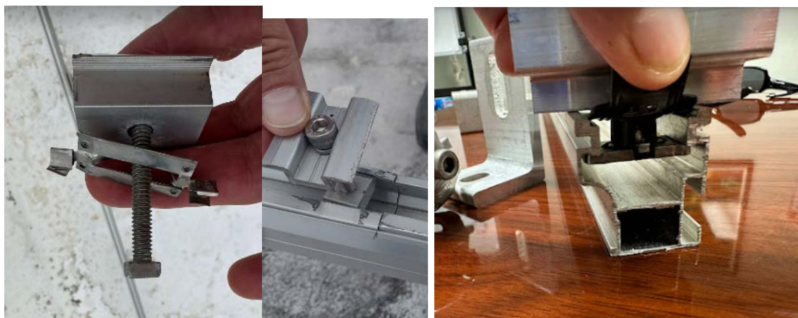
Figure 27. Some clamps have small bolt head (left) or nut (middle) contact area with the rail. These are prone to tearing out of the rail slot. Some products have significantly more contact area (right).
