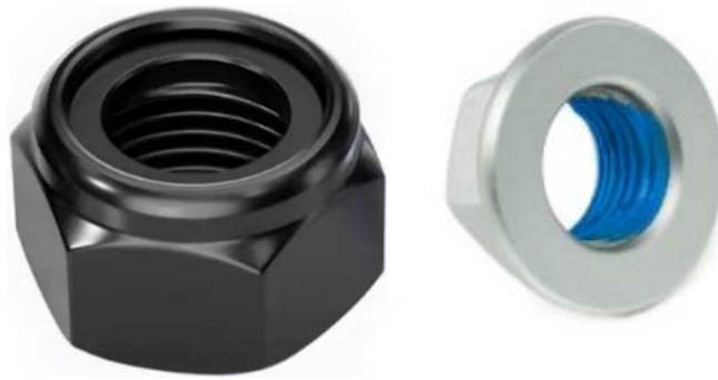
Figure 38. Two types of nylon nuts that can be used to resist loosening. Left is a prevailing torque nylon-insert nut. Right is a flange nut with pre-applied nylon patch.
