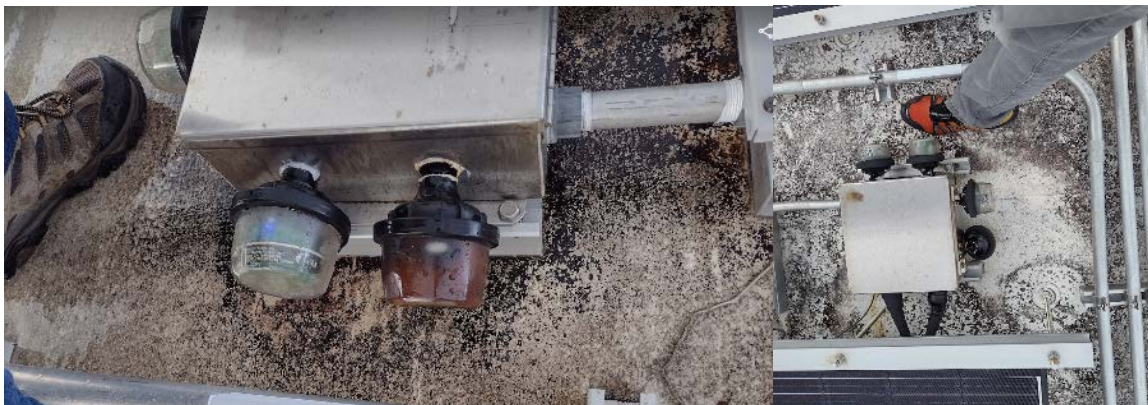
Figure 55. Failed DC surge protection devices with signs of water ingress and burnt components
