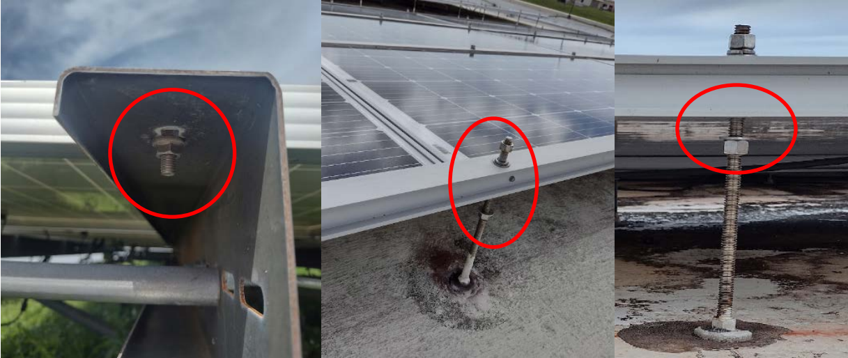
Figure 37. Bolts on PV systems can loosen over time. Locking hardware can help resist this loosening.
