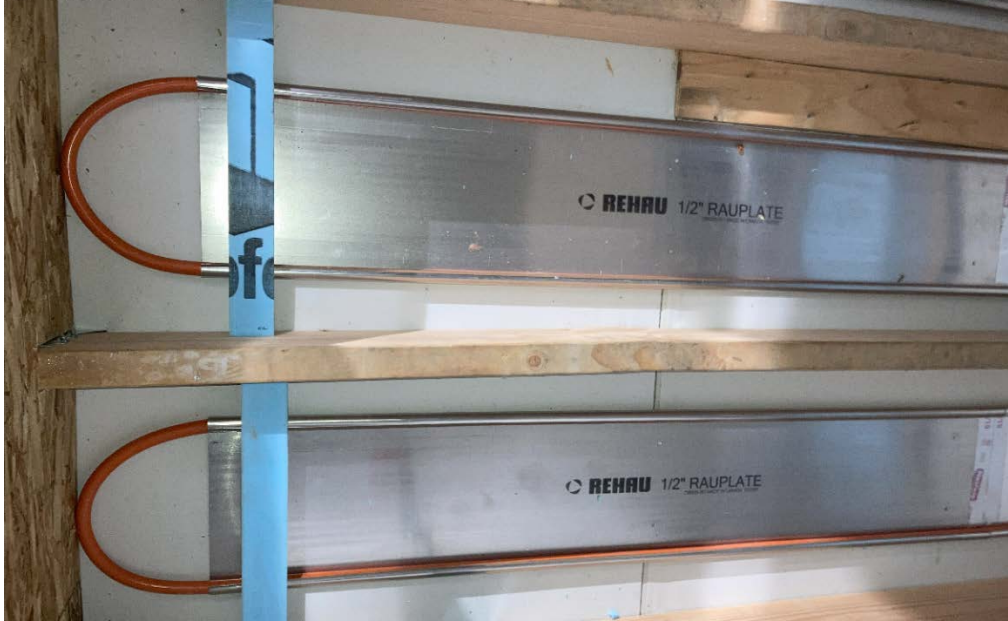
Figure ES-2. Site-built radiant ceiling panels used in laboratory tests
