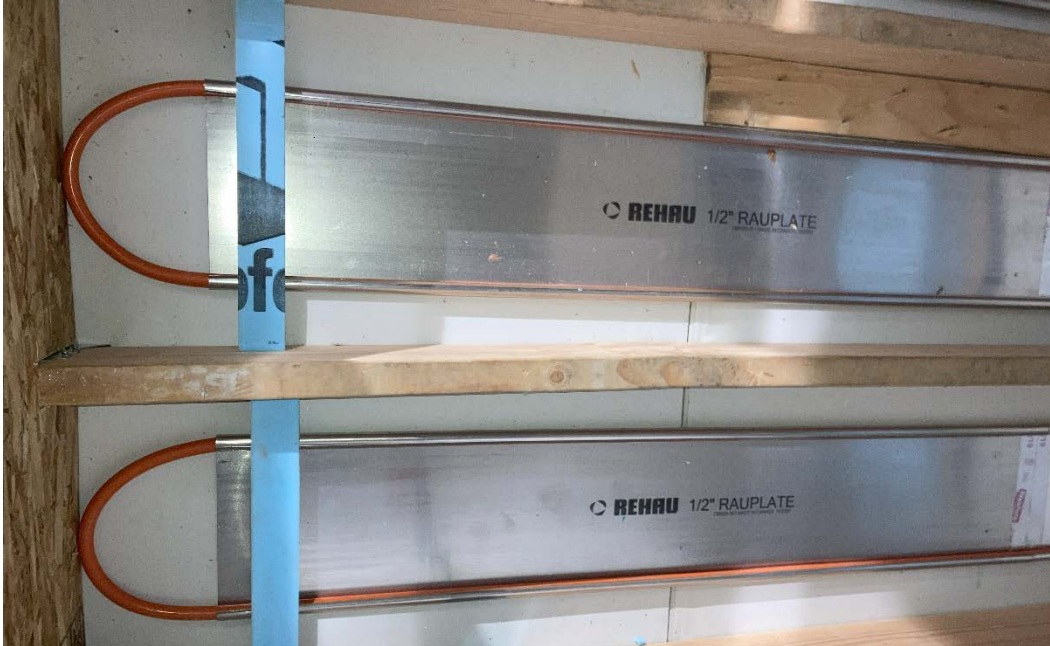
Figure 2. Site-built ceiling panels used in laboratory tests
