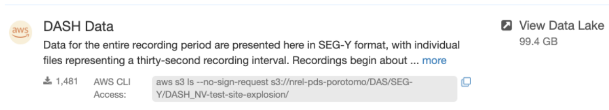
Figure 2: Example of a direct access link associated with a GDR data lake resource. Users can use the icon to the right to quickly copy the command so that they may paste it into their terminal for AWS CLI access to the data.
