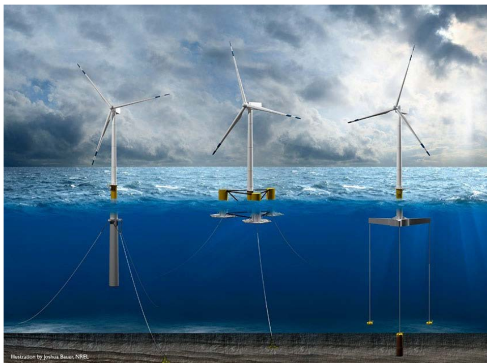
Figure 6. Types of floating OWTs, from left to right: spar-buoy, tension leg and barge stabilization concepts
