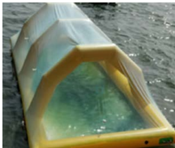
Figure 20. Example floating PBR device that uses wave energy to mix its microalgae culture solution 98
