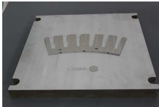
Figure 42. SLM multimaterial printed Fe 3 Si premixed with Al alloy using the 15-kW Bergey generator stator design.
