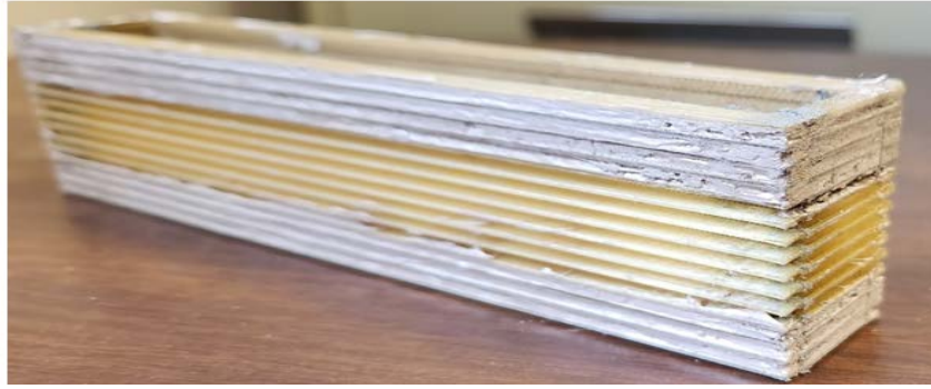
Figure 59. A sleeve (ULTEM 1010, two-part FFF option) partially filled with the AgCu0204-12 paste
