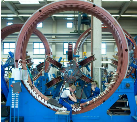
Figure 2. Winding process in a synchronous wind turbine generator.
