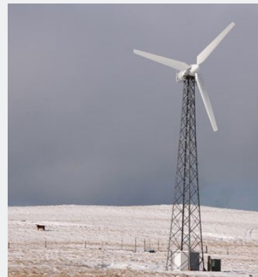
Figure 2. Nikolski installed a 65-kW remanufactured Vestas V-15 in 2007. Photo from Rich Stromberg, University of Alaska Fairbanks
