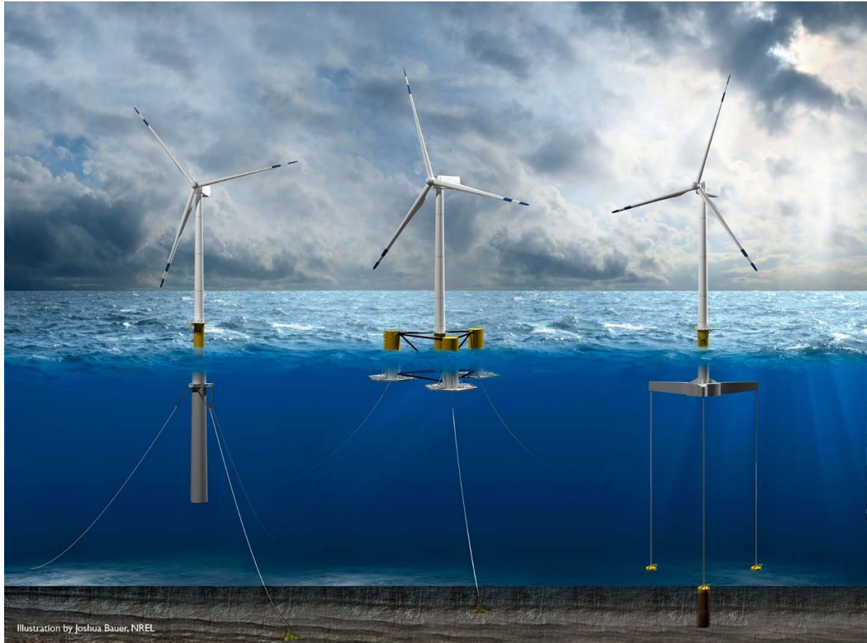
Figure 11. Three floating offshore wind energy substructure designs (left to right): spar, semisubmersible, and tension-leg platform.
