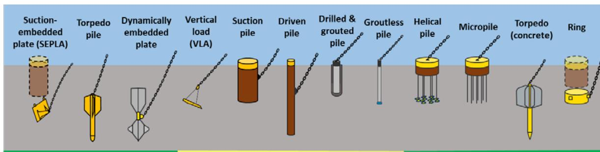
**Figure 25. Suitable anchor types for ultradeep water applications**
