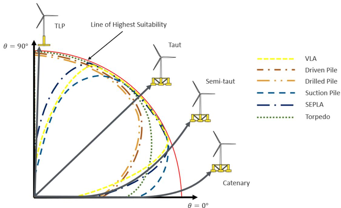
**Figure 24. Mooring load direction relative suitability for different types of anchors**
