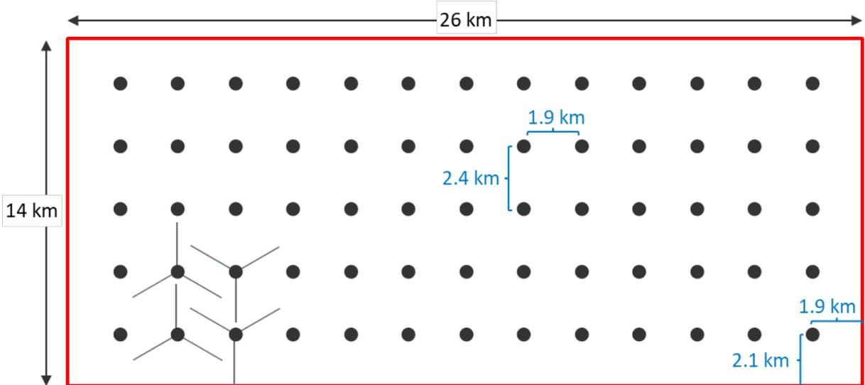
**Figure 53. Baseline plant layout at 3,000-m water depth**
