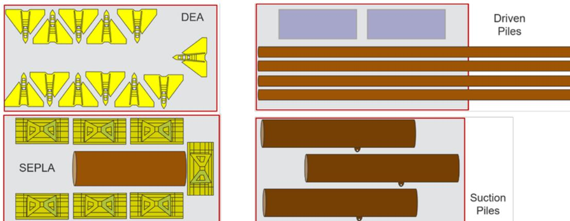
**Figure 21. Typical installation vessel deck layout for anchors**
