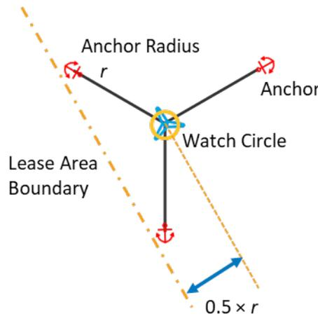
**Figure 42. Depiction of minimum distance from wind turbine position to lease area boundary**
