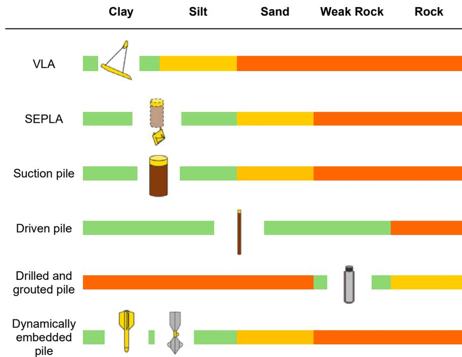
**Figure 20. Ground compatibility for suitable established anchor types in ultradeep water.**
