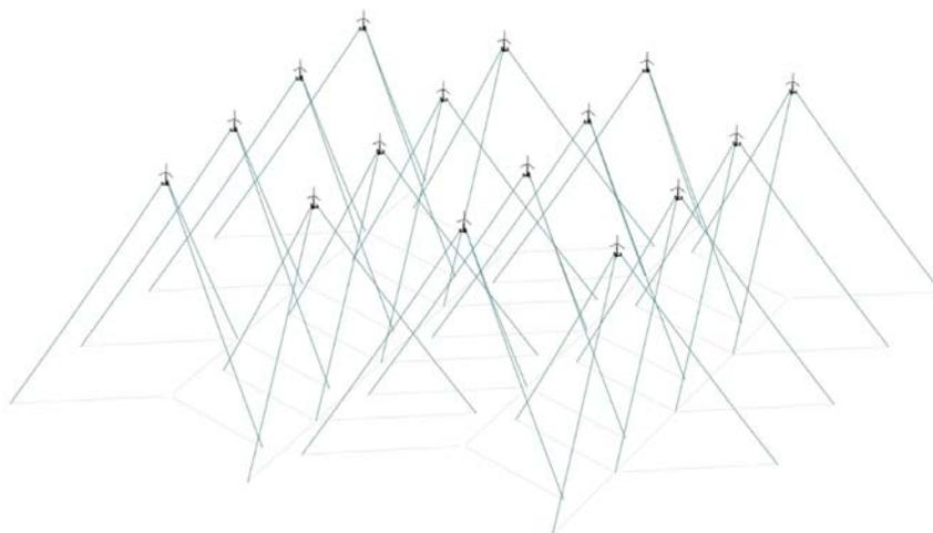
**Figure 40. Array of semisubmersibles with reference taut polyester mooring systems at 3,000 m water depth**
