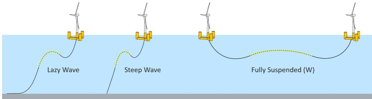
**Figure 6. Three common dynamic cable profile shapes**
