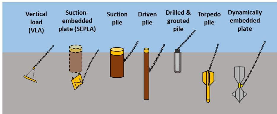
**Figure 18. Established anchor types suitable for ultradeep water**
