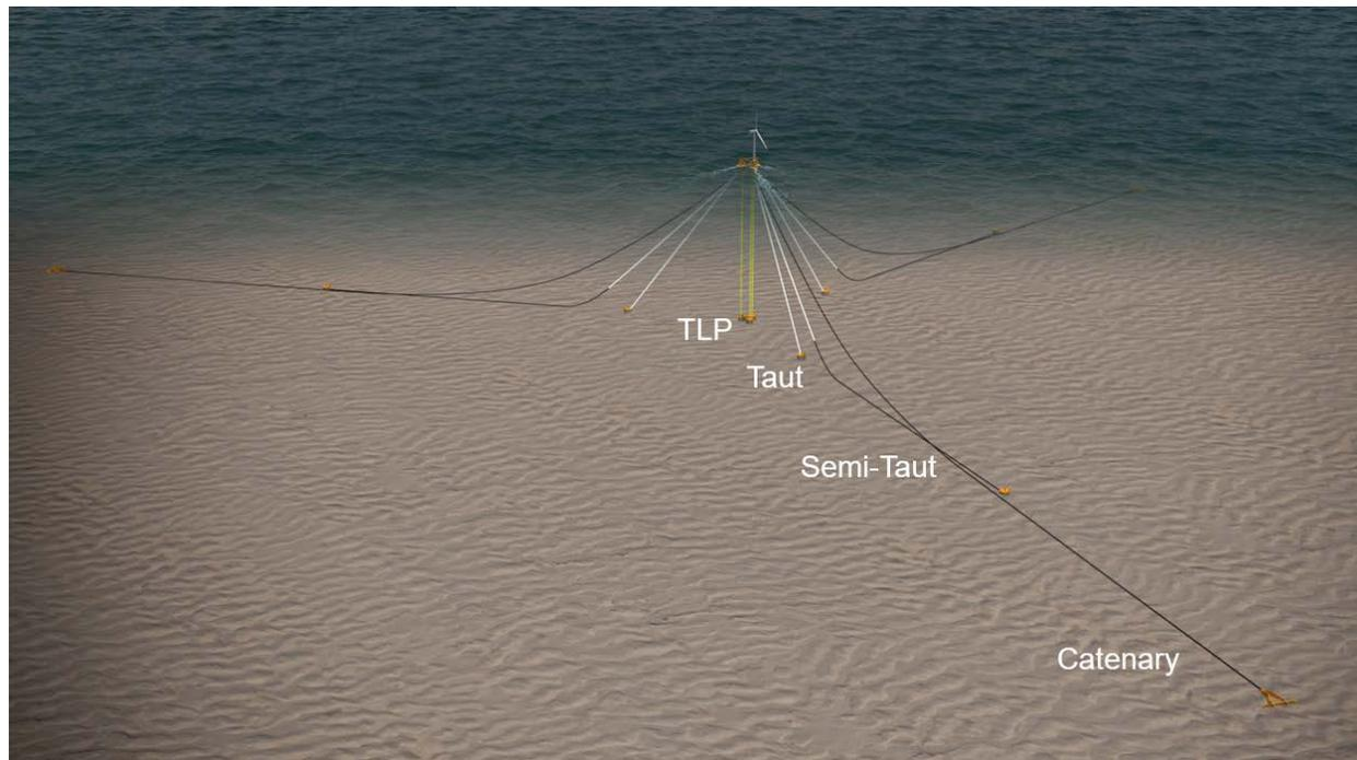
**Figure 3. Examples of mooring system configurations to scale relative to each other.**
