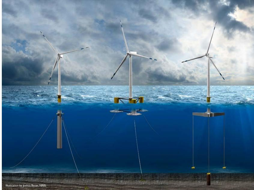
**Figure 1. Common floating support structure types for floating offshore wind. From left to right: spar, semisubmersible, and tension-leg platform.**
