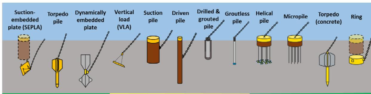
Figure ES-1. Suitable anchor types for ultradeep offshore wind applications
