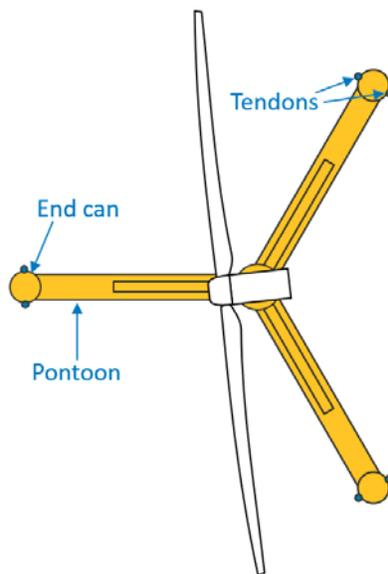
**Figure 35. Top view of TLP showing tendon positions**
