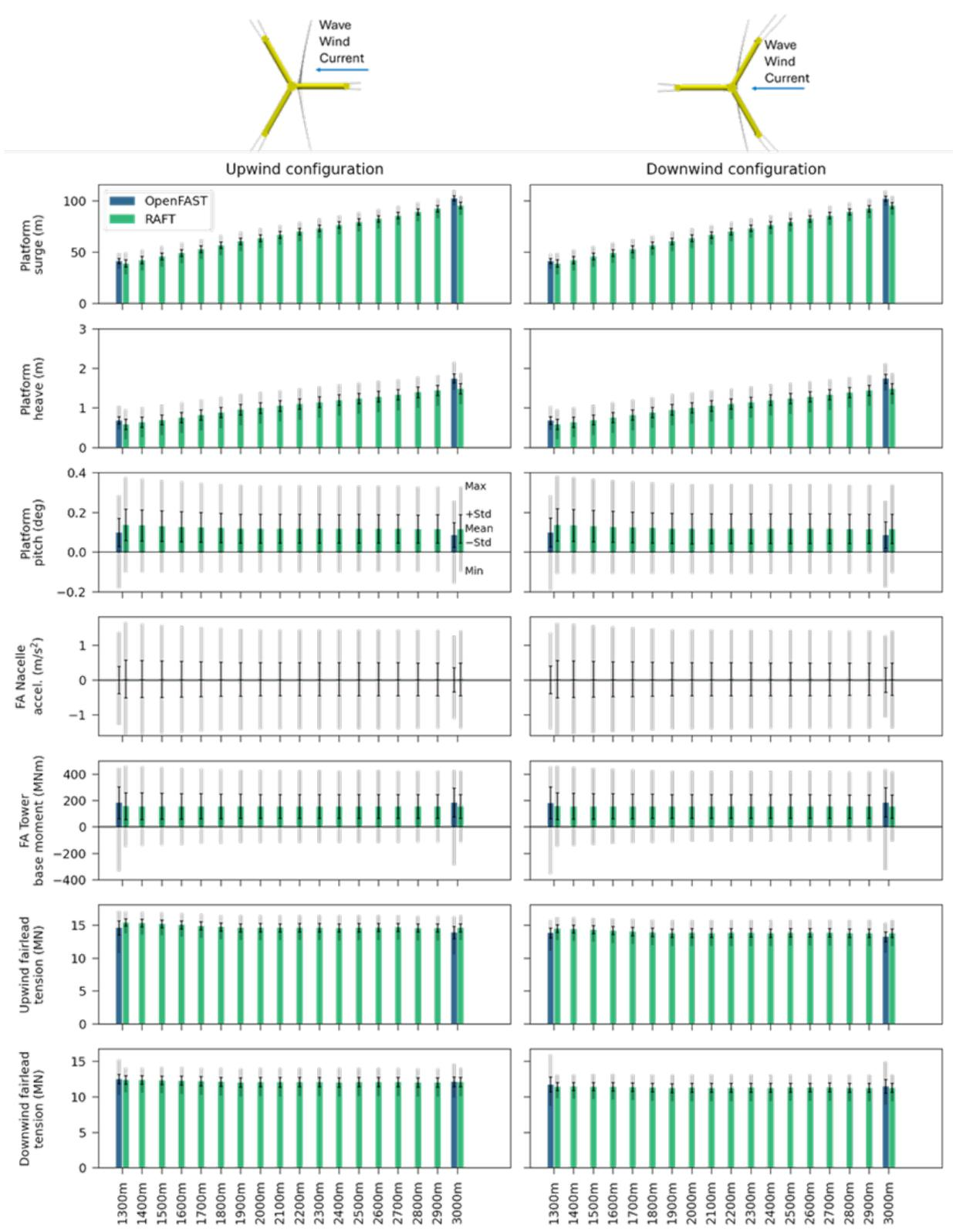
**Figure 37. Statistics of main quantities of interest obtained with RAFT and OpenFAST for DLC 1.6 for two different pontoon alignments with respect to the waves, wind, and current**
