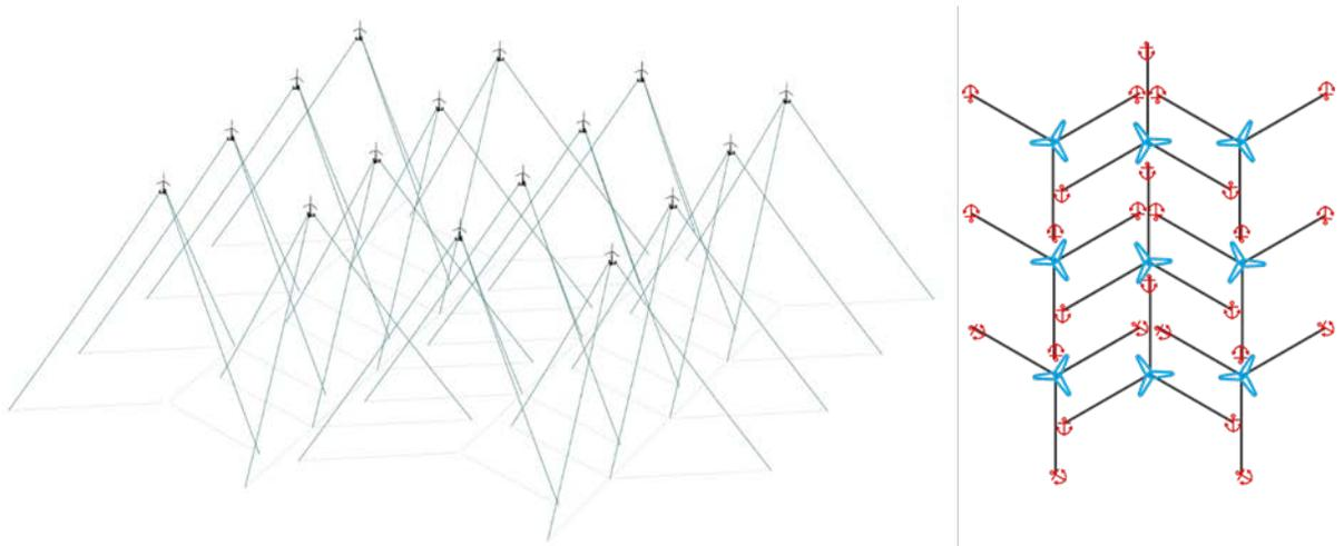
**Figure ES-6. (Left) Array of semisubmersibles with reference taut polyester mooring systems at 3,000-m water depth; (right) top-down view of array highlighting wind turbine positions (blue), mooring lines (black) and anchors (red)**
