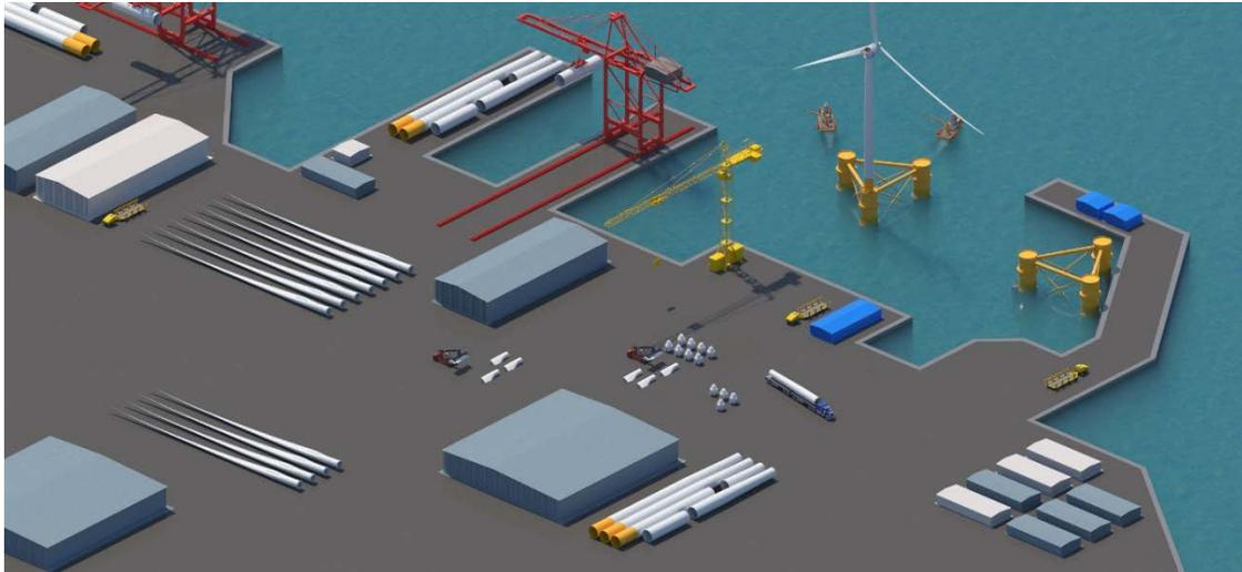
**Figure 7. A schematic of an example offshore wind energy port supporting floating wind turbine deployment.**
