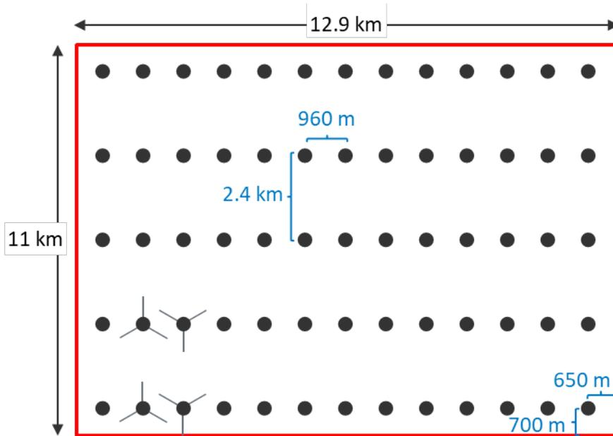
**Figure 52. Baseline plant layout at 1,000-m water depth**
