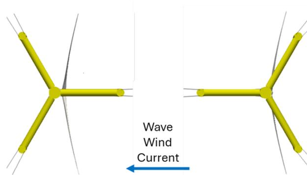
**Figure 36. Platform configurations with the pontoon aligned with the wave, wind, and current in an upwind (left) and downwind (right) orientation, viewing from below**
