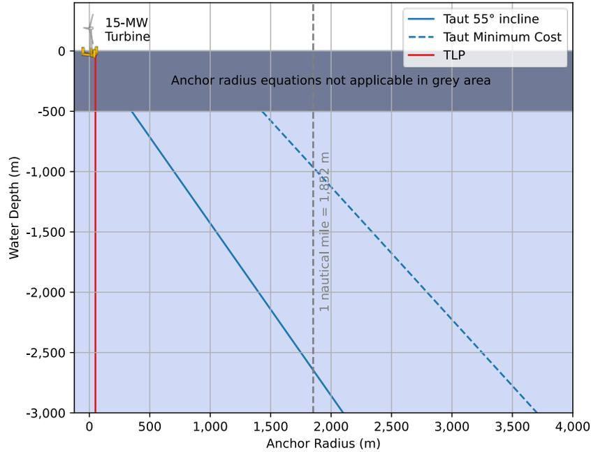
**Figure 41. Illustration of anchor radii for TLP and taut mooring configurations**
