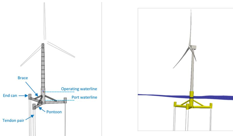
**Figure 34. Selected TLP topology for reference design**
