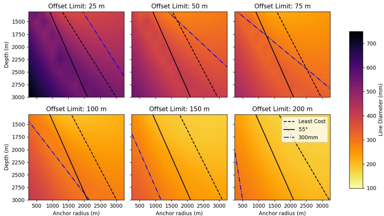
**Figure 31. Nylon taut mooring system diameters**
