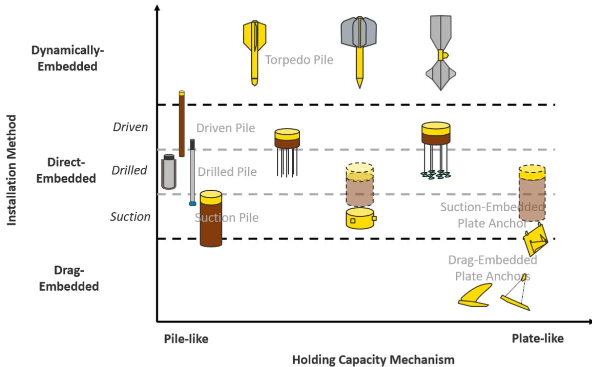
**Figure 17. Anchor types overlaid on a two-dimensional categorization by capacity mechanism and installation method**
