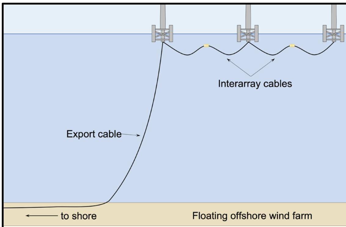
**Figure 10. An illustration of how electrical cables may be used at floating offshore wind farms. Inter-array cables connect between individual turbines and the combined energy is transported to shore with an export cable.**
