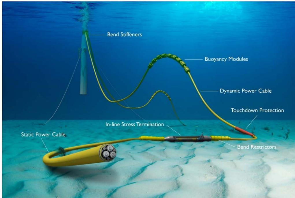
**Figure 5. Dynamic subsea cable system components.**
