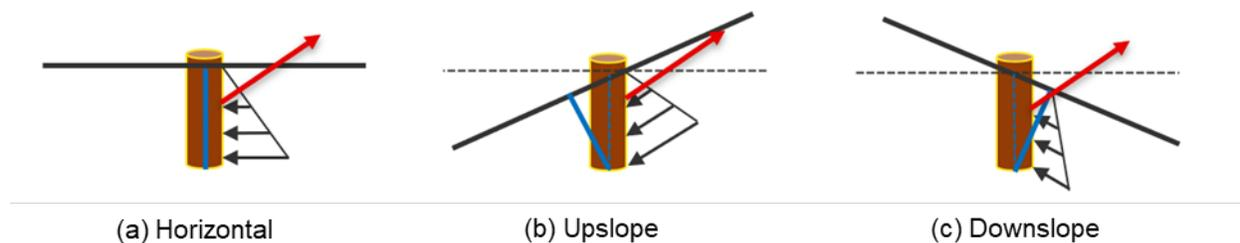
**Figure 19. Anchor holding capacity effects in a sloped seabed**
