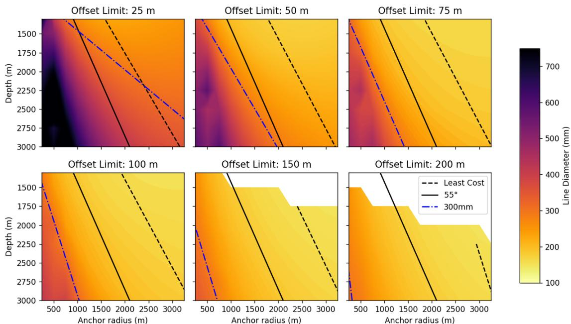
**Figure 29. Polyester taut mooring system diameters**
