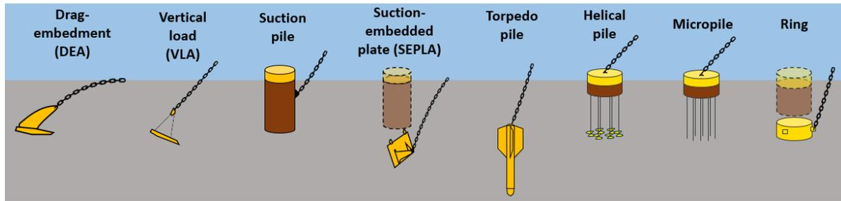
**Figure 4. Anchor technologies for offshore wind energy.**
