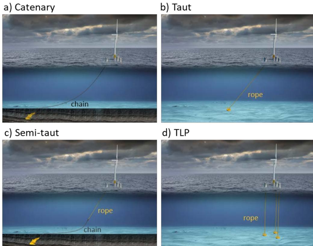
**Figure 2. Four common mooring line configurations.**
