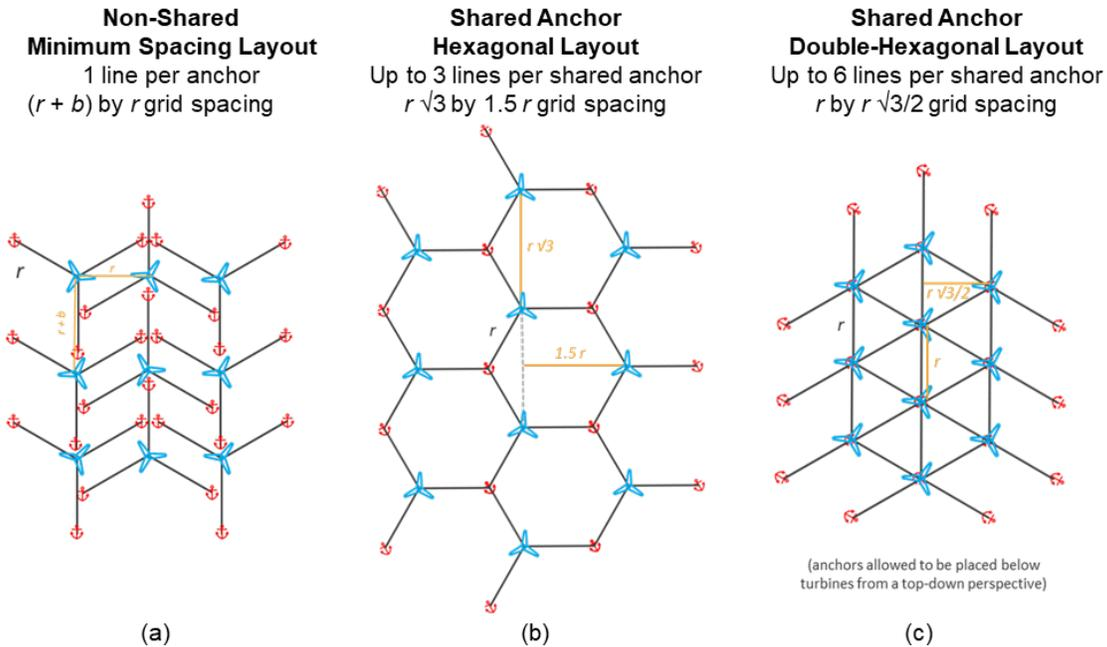
**Figure 43. Minimum spacing between watch circle centers for wind plant layouts with (b, c) and without (a) shared anchors. Blue rotor icons indicate watch circle centers and red anchor icons indicate anchor positions.**
