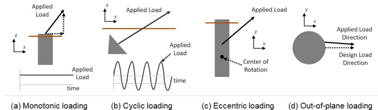
**Figure 23. Depictions of loading conditions that an anchor can experience**
