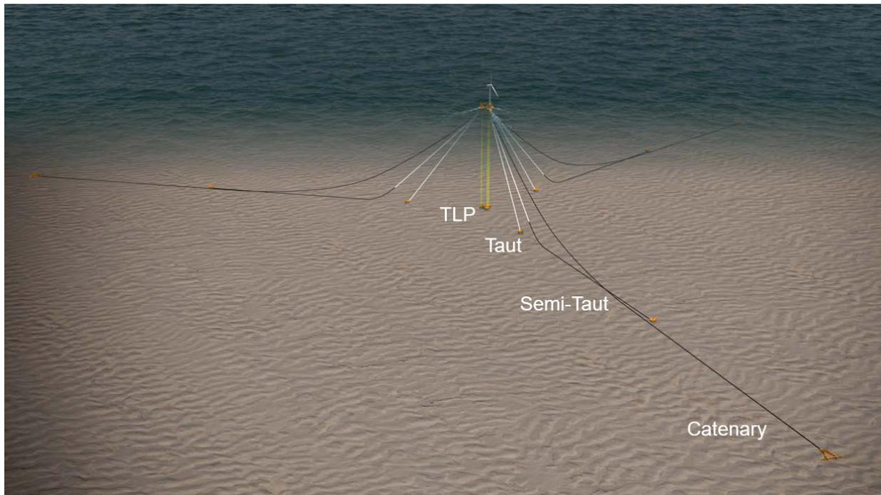
**Figure ES-2. Mooring system configurations showing relative seabed area required for each type**
