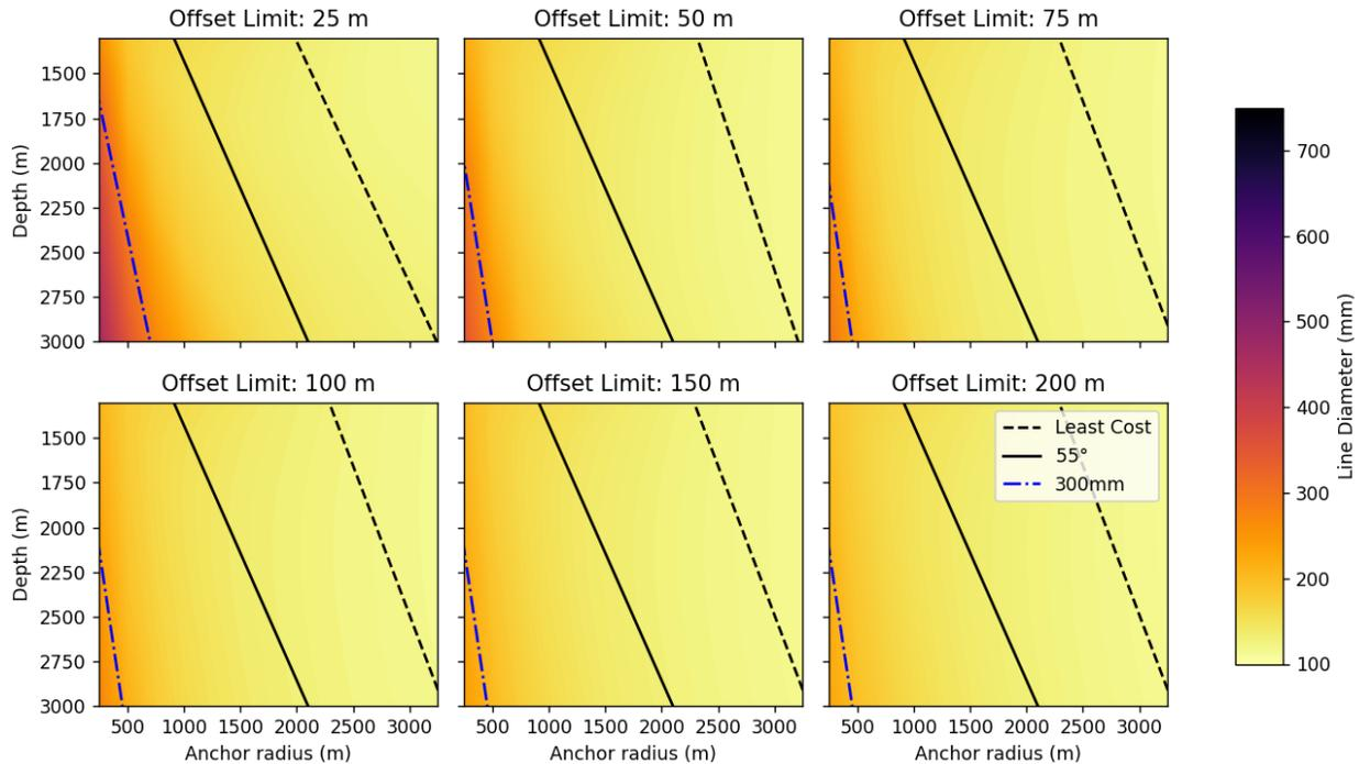
**Figure 33. HMPE taut mooring system diameters**
