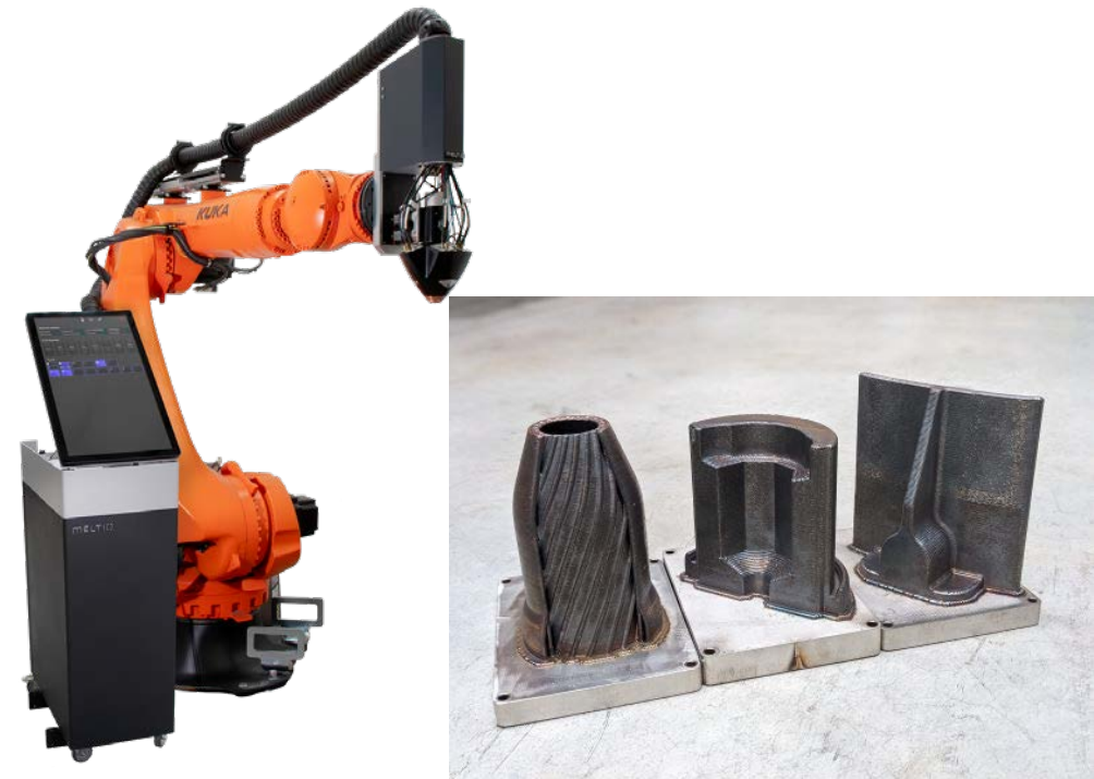
Wire-Laser Metal 3D Printing
