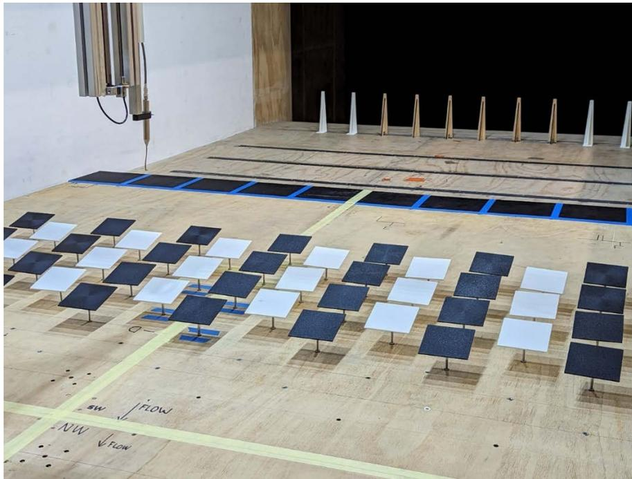
**Figure 23. Linearly staggered array of heliostat models instrumented with three-axis load cells and a multi-hole pressure probe and traverse system for flow characterization in the University of Adelaide wind tunnel**
