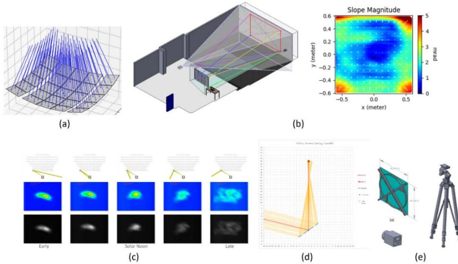
**Figure 9. A few OpenCSP examples. (a) Heliostat representation. (b) SOFAST 2.0 deflectometry system. (c) BCS dataset spanning daily and annual variation. (d) Interactive ray-trace tool. (e) CAD examples.**
