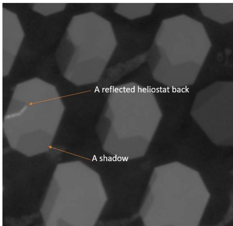
Figure 40. Cropped image from Heliogen field camera of several heliostat mirrors when specifically posed relative to field geometry and solar direction
