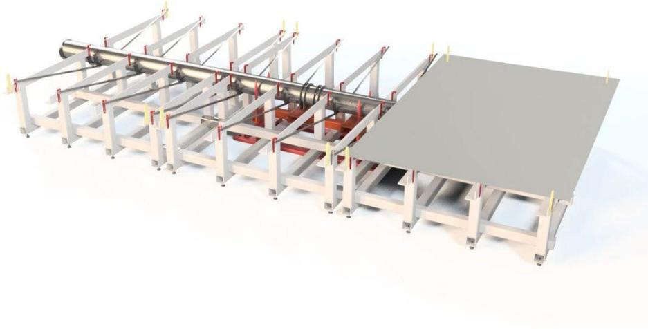
**Figure 30. CAD model of mirror array workstation prototype with one facet placed. Sixteen vertically adjustable control points (highlighted in red) per facet allow 2D focusing of the mirror array.**
