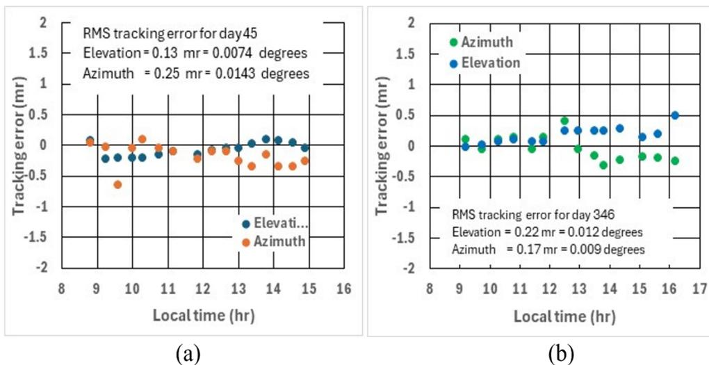
**Figure 43. Sandia tracking tests of McDonnell Douglas heliostat #1 in 1983**
