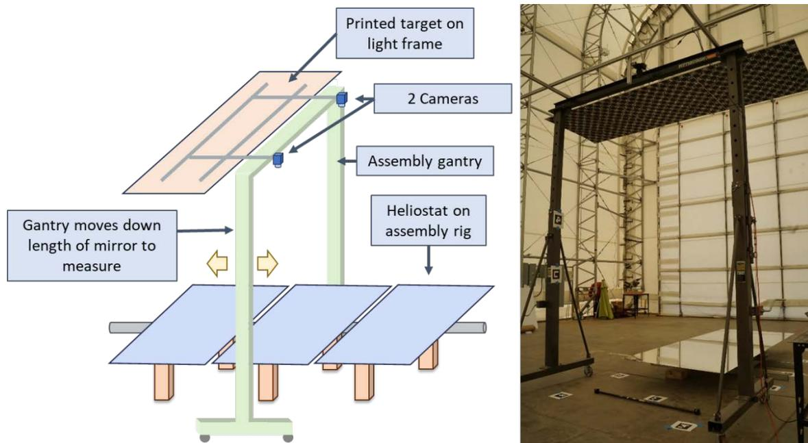
**Figure 50. A unique ReTNA layout, specific to Solar Dynamics’ heliostat assembly. Diagram of the design (left) and image of initial installed system (right).**
