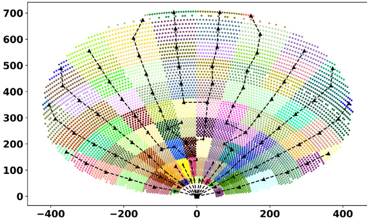
Figure 31. Data traffic routing to the central station based on the least path loss-based routing algorithm for a daylong simulation (Jan. 1, 2020) based on real data.
