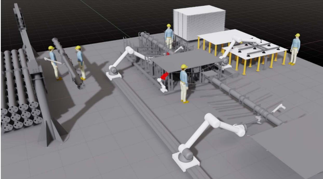
**Figure 38. Digital twin of a heliostat manufacturing facility. The digital twin enables the users to view how the humans and robots are performing the assembly with the expected timing. Optimization of the position of each station, robot, and operator can be done with the simulation within the digital twin.**
