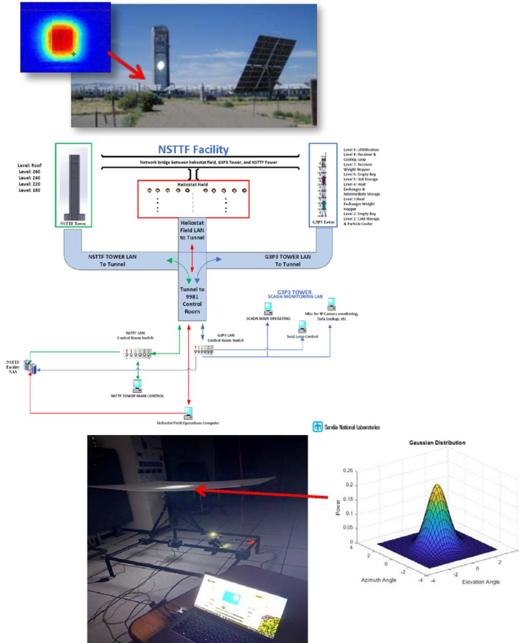
**Figure 13. Top: Sandia National Solar Thermal Test Facility (NSTTF) solar tower with on-sun beam and BCS metrology image, used for feedback controls. Middle: Sandia NSTTF closed-loop control system architecture. Bottom: Laboratory closed-loop controls testbed for controls screening with a smaller target.**
