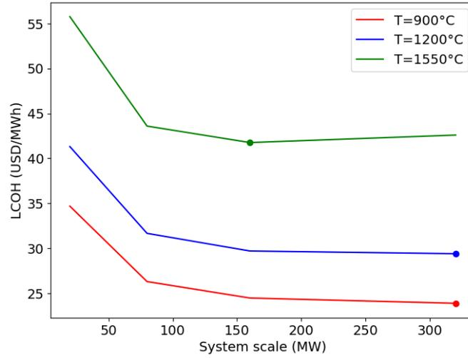
**Figure 28. Optimal LCOH as a function of system scale for three high-temperature applications**
