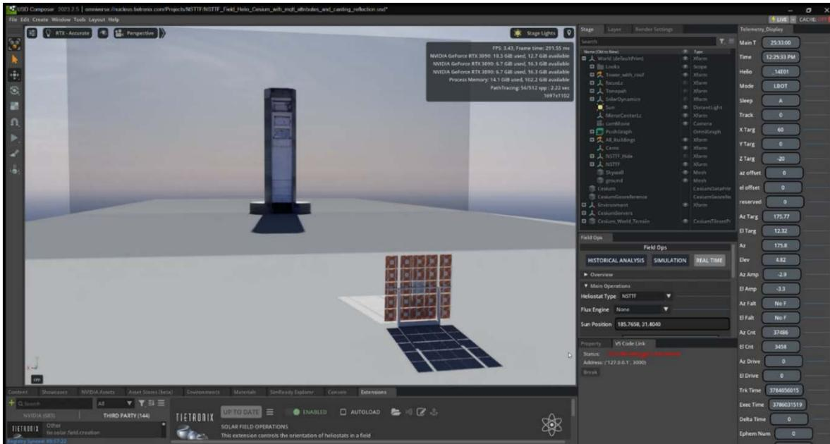
Figure 36. Digital twin of one heliostat at the NSTTF, playing back the log file of an experiment operation. The digital twin provides visualization of the heliostat motion and displays the telemetry data captured during the experiment.
