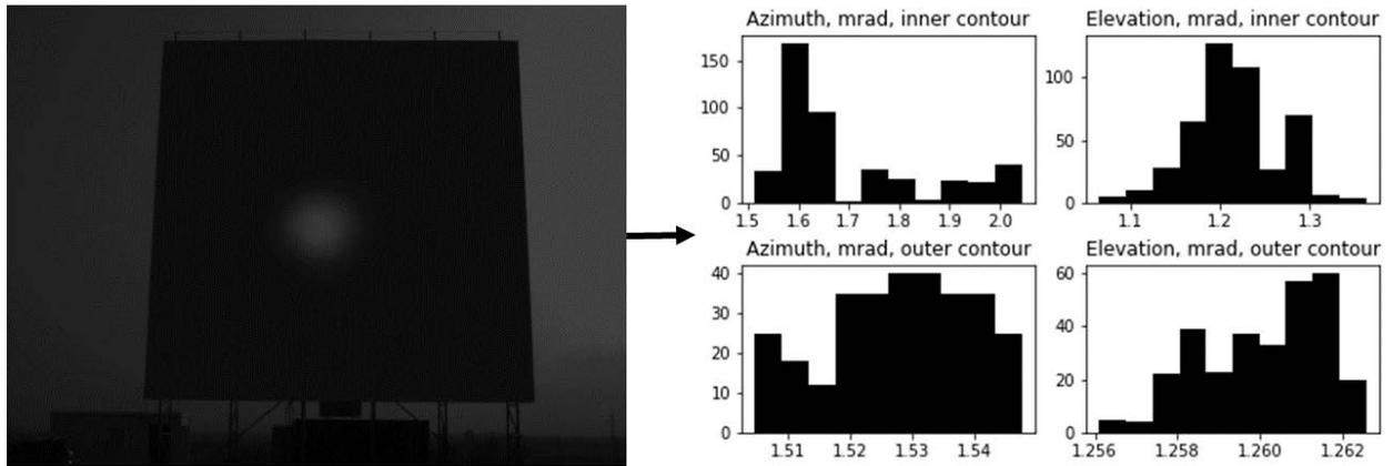
**Figure 48. Left: One raw BCS image from a round robin partner institution’s contribution to the shared dataset. Right: NREL preliminary sensitivity study result of varying image preprocessing parameters on this particular image, with the y-axis representing the number of preprocessing parameter combinations resulting in the calculated tracking deviation indicated on the x-axis. Two image post-processing methods are used: inner contour and outer contour.**
