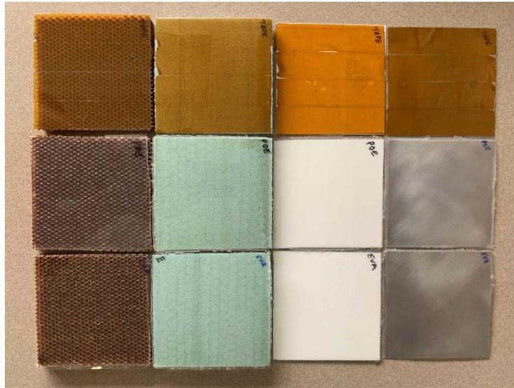
**Figure 11. The nine different combinations of surface and adhesive materials subjected to peel testing**
