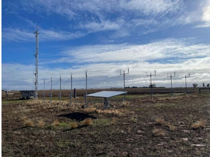
**Figure 24. ABLRF: heliostat model instrumented with a load cell and pressure sensors, and horizontal and vertical arrays of ultrasonic anemometers for ABL turbulence measurements**
