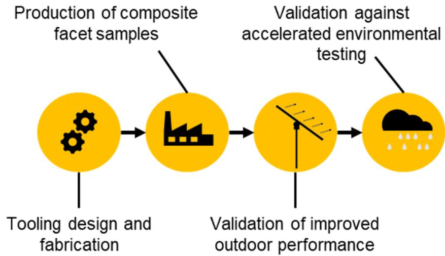
**Figure 51. The overall plan for developing and testing composite facets that are consistent with HelioCon goals for low-cost heliostats**
