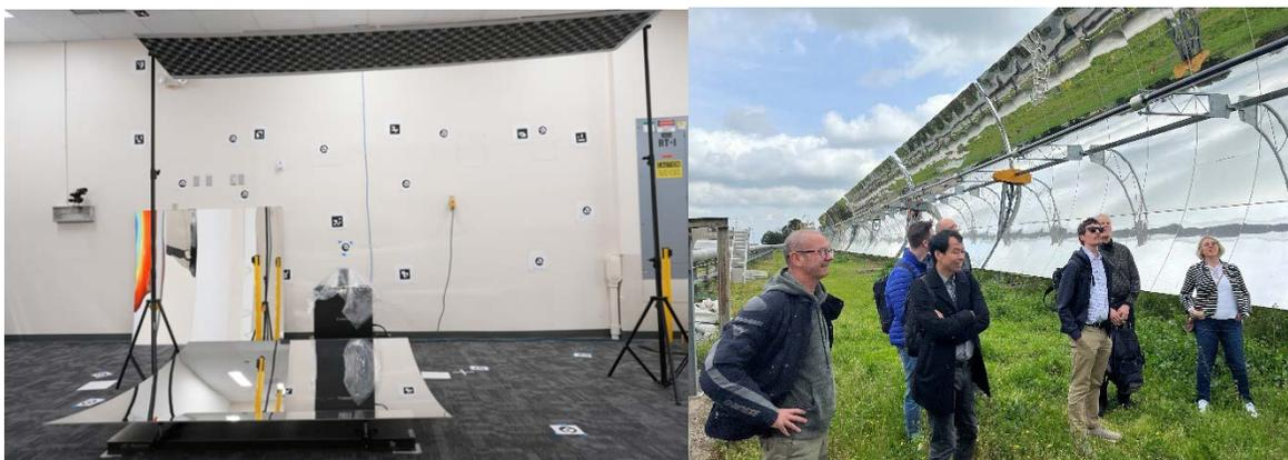
**Figure 47. Right: Measurement of a round robin trough facet at Sandia. Here, a portable ReTNA target is set up underneath Sandia’s SOFAST target screen. Left: Participants in the SFERA-3 round robin project at ENEA.**
