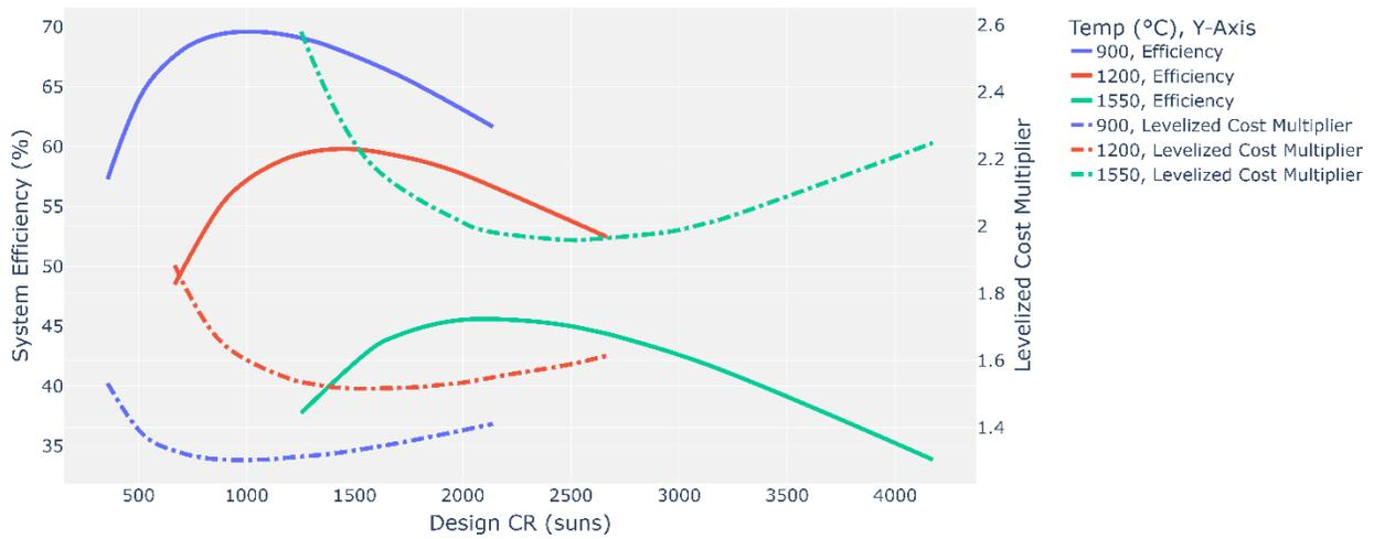
**Figure 19. System efficiency and relative LCOH as a function of design concentration ratio for a case study with a 160-MW<sub>th</sub> receiver operating at 1,200°C**
