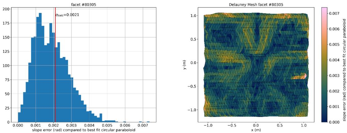
Figure 22. Example of analysis result. Left: Histogram of slope errors and RMS area-weighted slope error. Right: 2D plot of meshed point cloud colored by slope error of each facet, compared with best-fit paraboloid (CSIRO).
