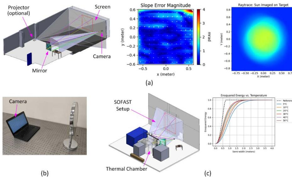
**Figure 7. Example SOFAST applications. (a) Single heliostat facet with ray-tracing analysis. (b) Laptop installation for education. (c) Thermal chamber setup and temperature analysis.**
