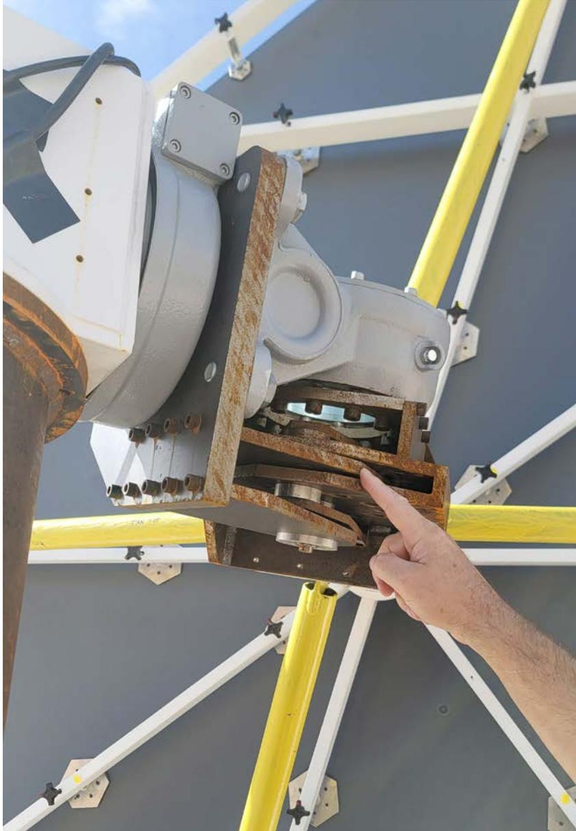
**Figure 35. The twisting heliostat is purely mechanical: No computer is required**
