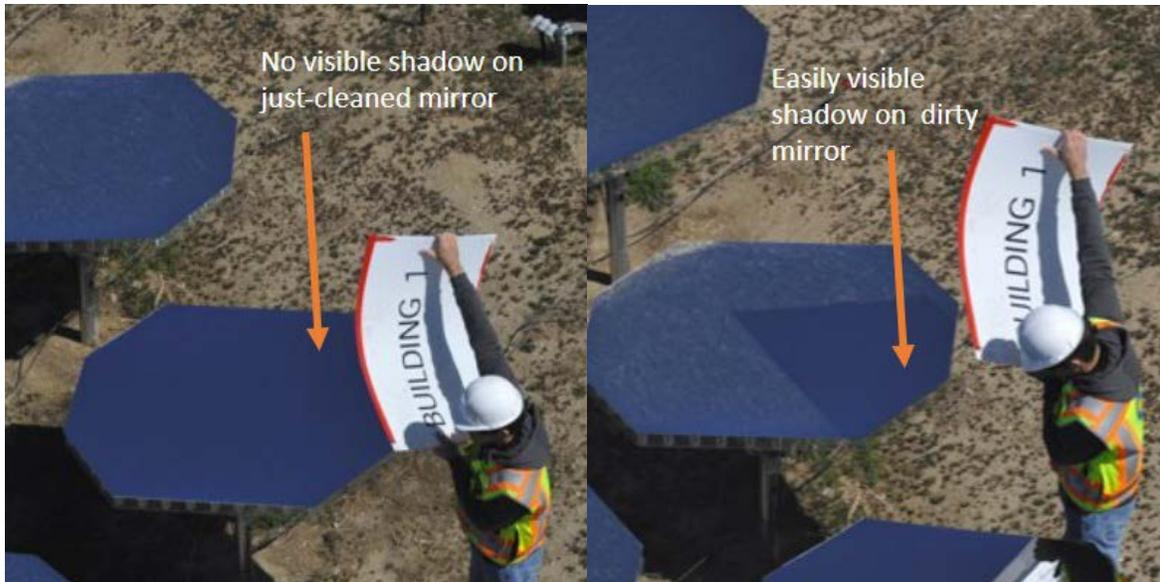
Figure 39. Clean (left) and dirty (right) mirrors. Shadow is visible on soiled mirror but not on clean mirror.
