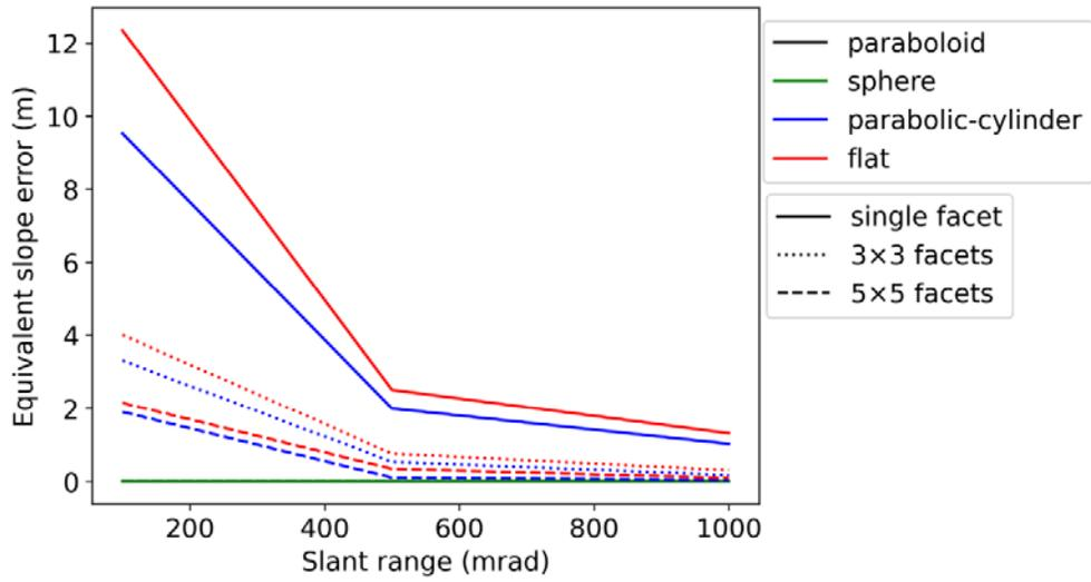
**Figure 27. Equivalent slope errors of 12 configurations of heliostats**
