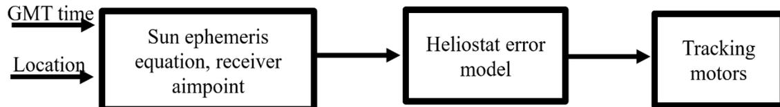
**A heliostat error model was used to modify the tracking angles.**
