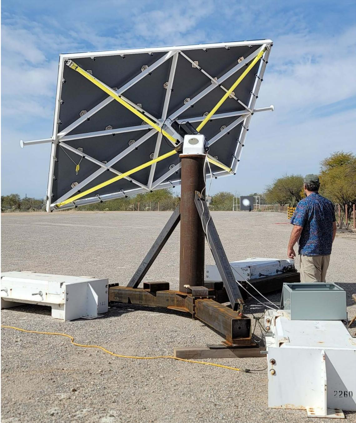
**Figure 34. A full disk image of the sun is reflected to a target (distant right) from a twisting heliostat**
