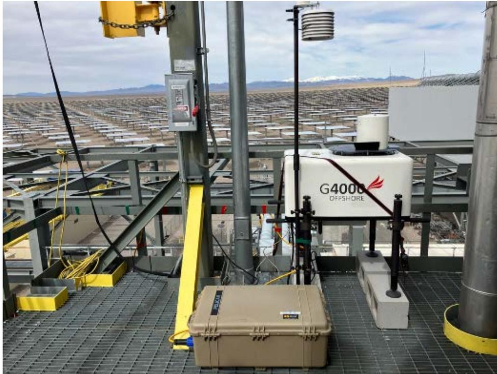
Figure 54. Lidar installation at Crescent Dunes
