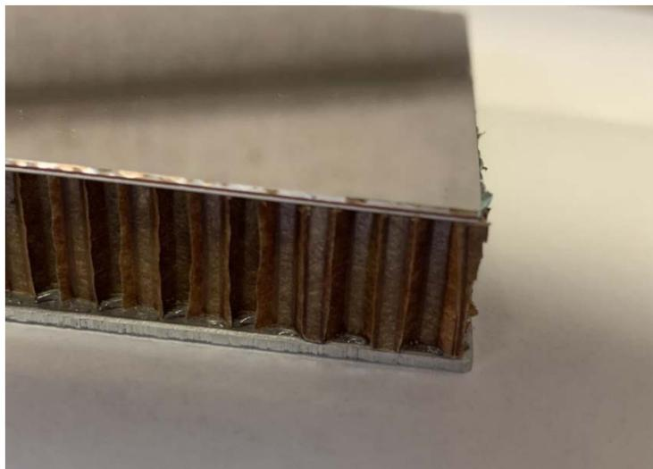
**Figure 12. A sample laminate stack with a 1- mm mirror supported by honeycomb before applying and edge seal structure**
