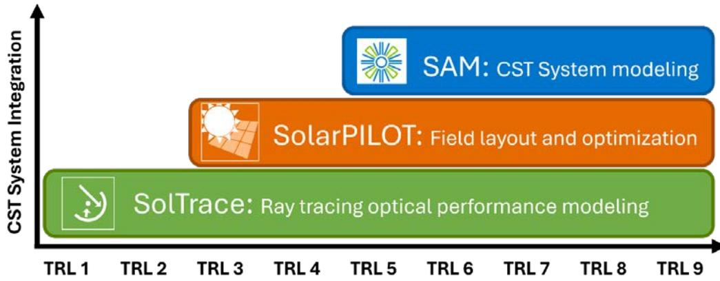
**Figure 56. SolTrace MCRT serves as the foundation of CST system performance modeling and enables optical characterization of novel collector and receiver designs**
