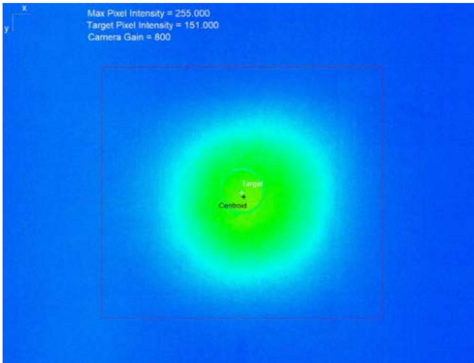
**Figure 58. First beam on tower using new software and graphical user interface with updates to minimize vibrations and keep the beam within 0.02 degrees of GPS timer**
