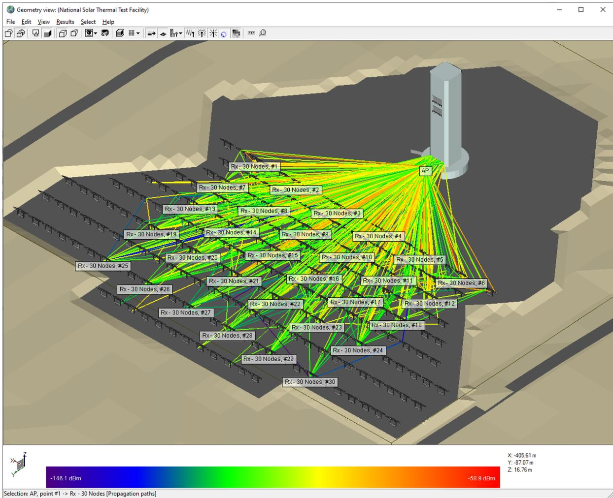
**Figure 32. Image of NSTTF 30-node wireless simulation visually indicating wireless signal path lost between access point radio and heliostat**
