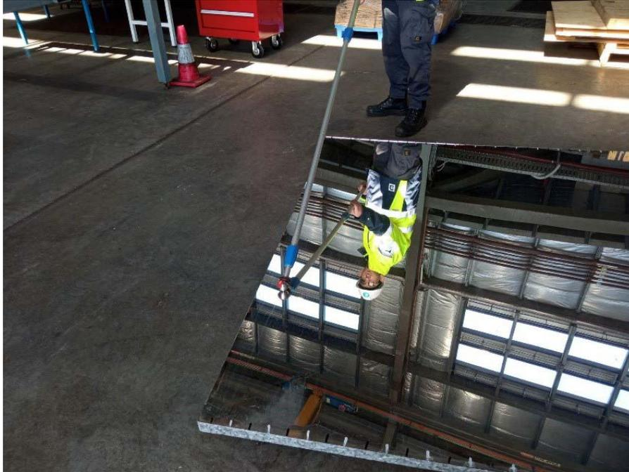
Figure 21. Using a laser tracking coordinate measuring machine (Leica AT901) to measure the heliostat surface point cloud (CSIRO)
