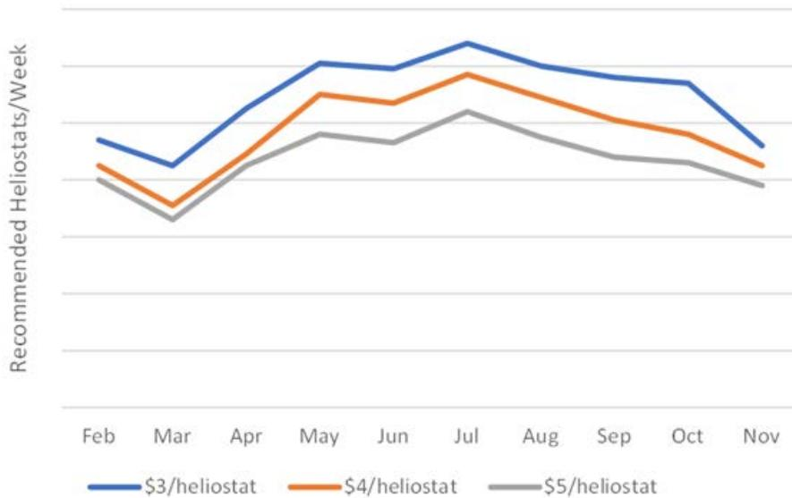
Figure 16. Monthly recommended cleaning schedule, in heliostats per week, for the Ivanpah facility, using the deterministic optimization approach and a fixed soiling rate of 0.1% per week for the field
