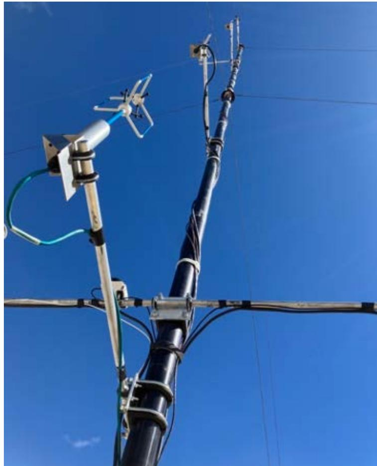
**Figure 53. The inflow tower and sonic anemometers installed at Crescent Dunes**
