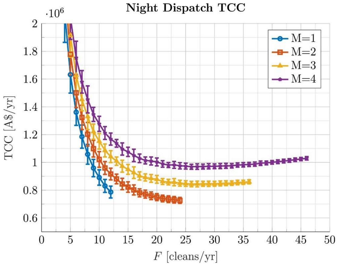
Figure 25. Total cleaning cost for a 56-MW plant equipped with modular solar fields in a nighttime dispatching scenario for varying numbers of cleaning crews
