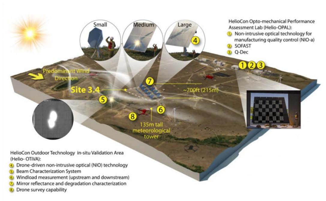
**Figure 6. An illustration of the third-party heliostat evaluation platform at NREL's Flatirons Campus**
