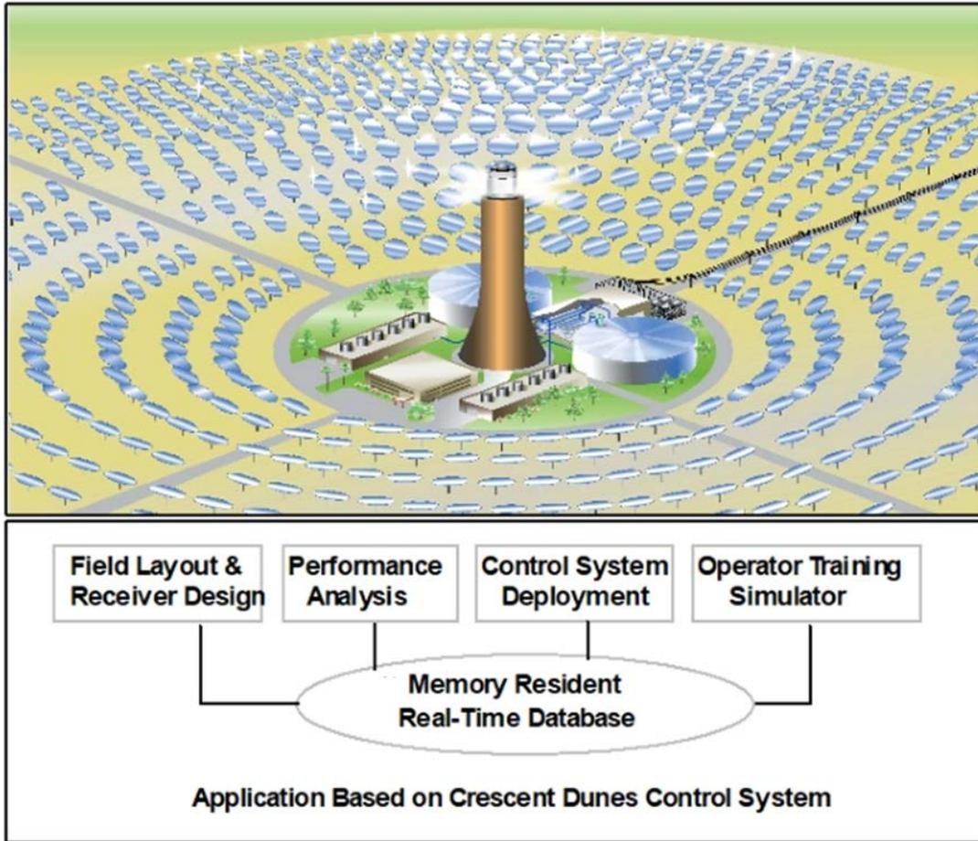
Figure 45. Diagram of generic heliostat field design and control system.
