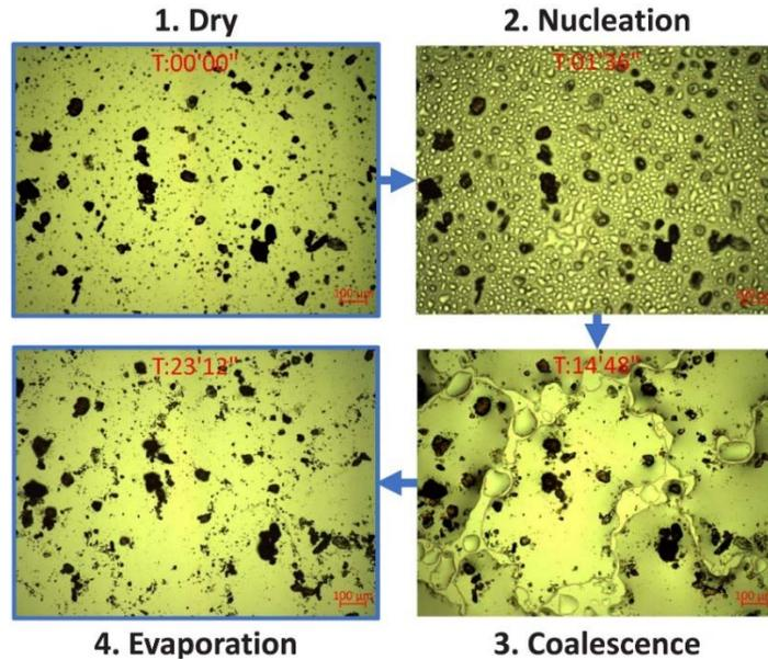
Figure 26. Bright-field microscope images of the four stages of moisture condensation on a cold mirror sample surface, magnification at 10x
