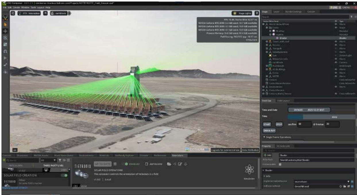
Figure 37. Visualization of the full NSTTF solar field, focusing on the receiver with the flux map computed with the fast ray-tracing simulation software
