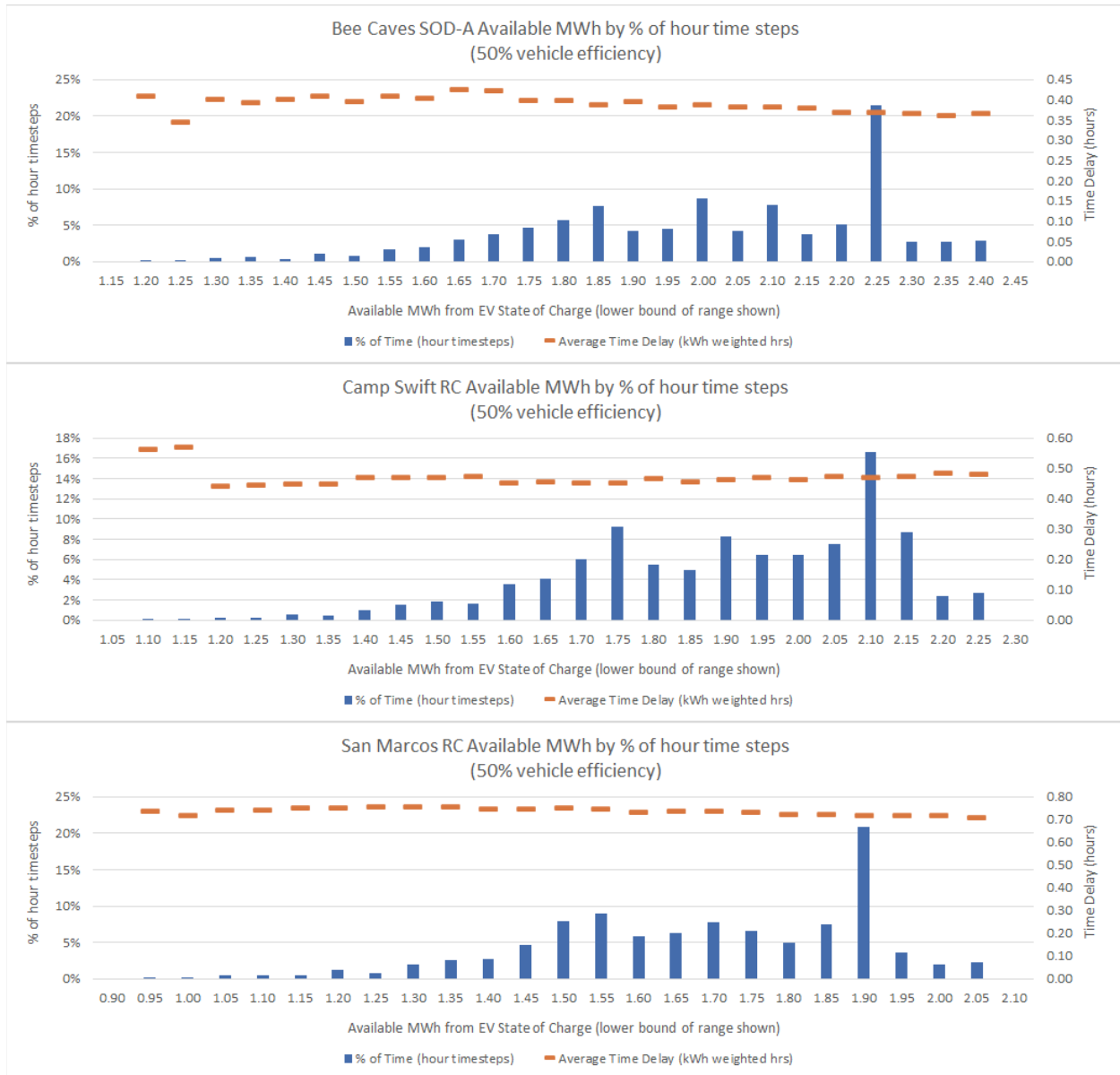
Figure 31. Distribution of all time steps showing energy available from nearby fleet vehicles if replaced with equivalent EVs operating at 50% efficiency
