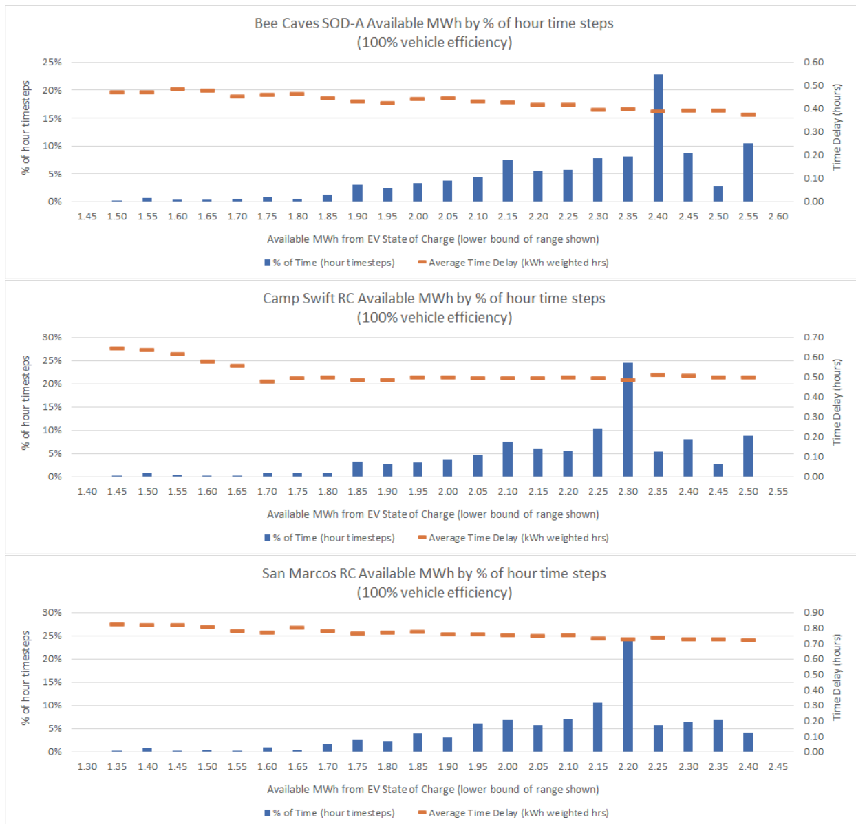
Figure 30. Distribution of all time steps showing energy available from nearby fleet vehicles if replaced with equivalent EVs operating at 100% efficiency
