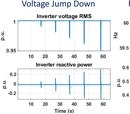
Reactive power responds correctly • to the voltage dip.
