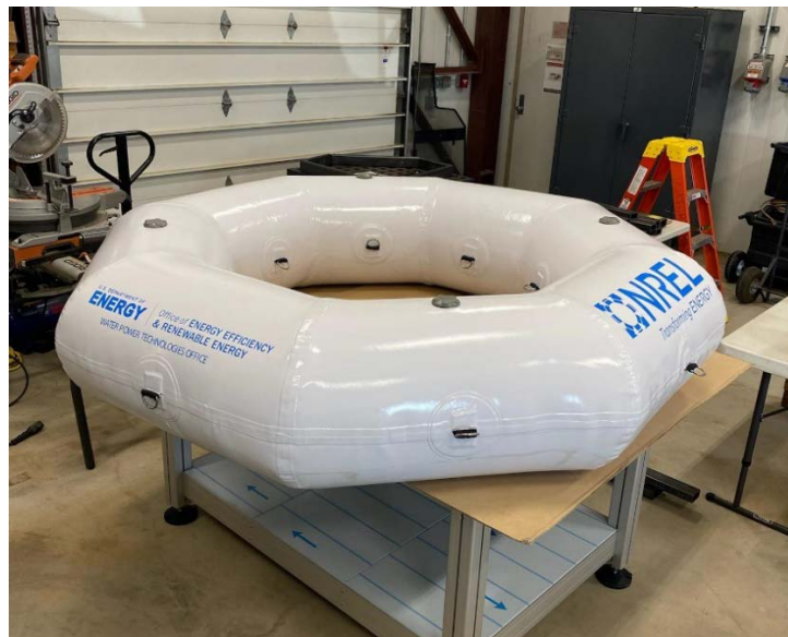
Figure 5. Inflatable four-chamber float used to provide buoyancy
