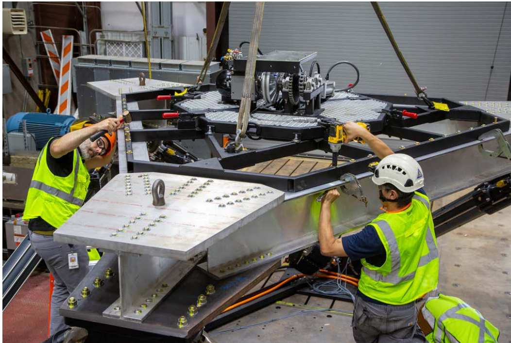
Figure 26. HERO WEC and adapter frame being secured to LAMP
