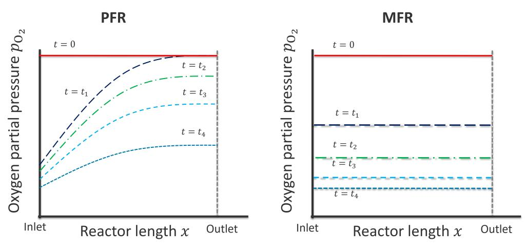
Unlike the MFR assumption, packed bed reactor undergoing chemical looping will exhibit chemical potential gradient
