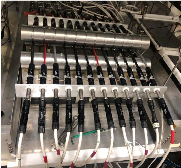
Figure 15: Initial image of C-AST dynamic fixture, with the unaged specimens in the formal experiment.
