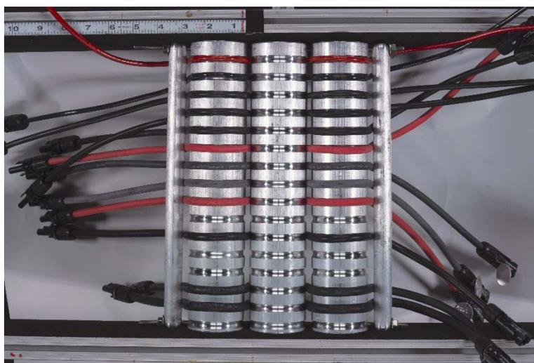
Figure 16: Initial image of K3, the 3rd C-AST kinematic fixture, with the unaged specimens in the formal experiment.
