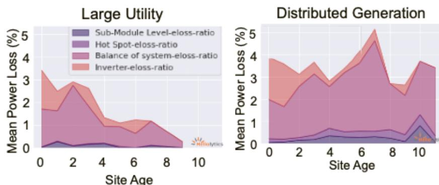
Figure 2: Comparison of the origin of power loss between PV installations of different size. The data, shown for BoS components (combined for cables, connectors, and fuses), comes from a site inspection service provider<sup>3</sup>.
