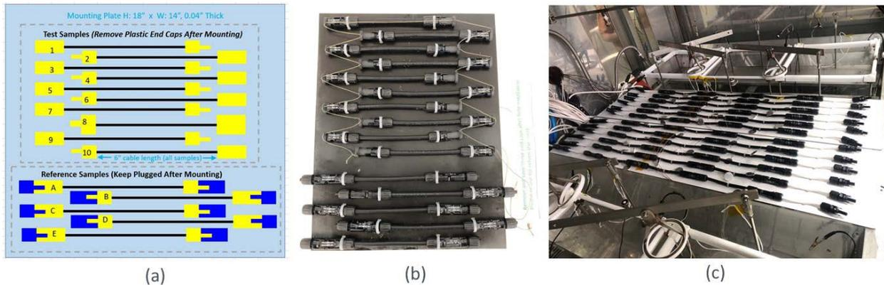
Figure 17: Uncapped connector experiment, including: (a) schematic of outdoor fixture, (b) photograph of the connectors in the outdoor fixture (in 1 x1 configuration, returned from Gaithersburg, MD), and (c) photograph of the connectors in the indoor C-AST fixture (after being assembled into 1 x 3 configuration). Specimens have already been returned and reexamined after outdoor aging in Barstow, CA; Gaithersburg, MD; and PEI, CAN and are presently in C-AST aging.
