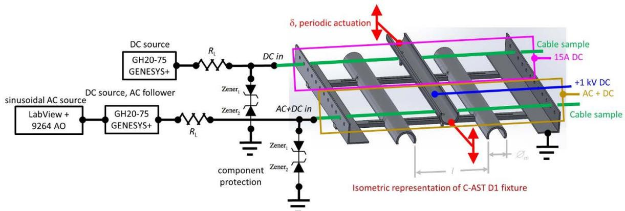
Figure 14: Schematic showing the additional features of the “dynamic” fixture (D1), including external perturbation in addition to direct current which may be superimposed with alternating current to simulate inverter switching noise. Key aspects of the electrical circuits are shown including sources, protective diodes, and electrical grounding.
