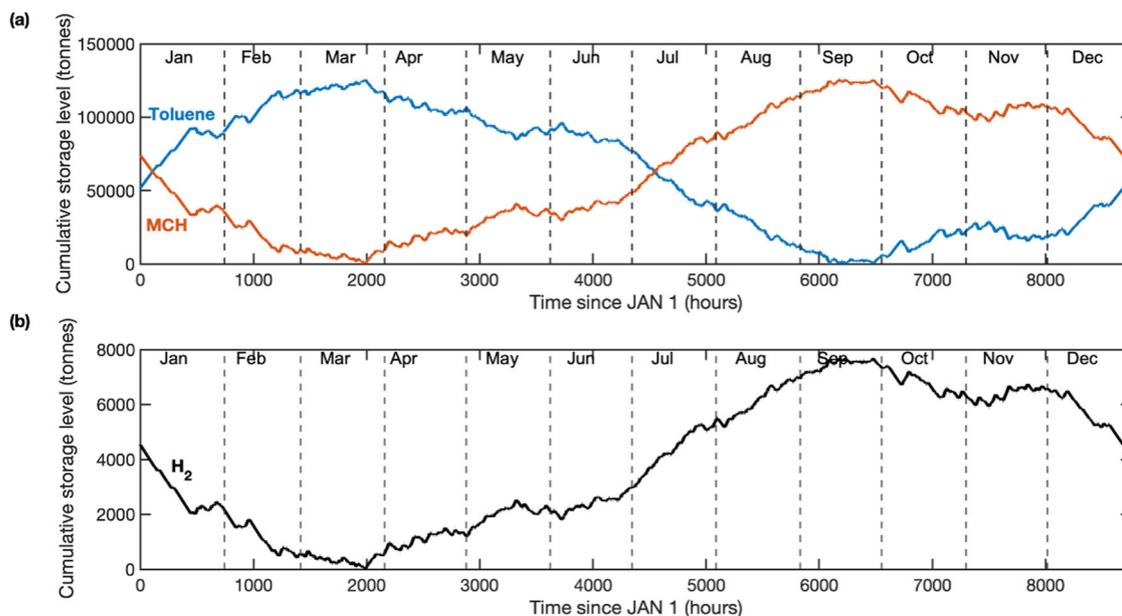
**Fig. 1 | Storage of hydrogen and corresponding tank fill levels for toluene and methylcyclohexane (MCH).** **a** Cumulative liquid storage of toluene versus methylcyclohexane over a sample year for a location with the median national levelized cost of storage of \$1.84/kg-H<sub>2</sub>. **b** Stored H<sub>2</sub>, which is equivalent to surplus or otherwise-curtailed H<sub>2</sub>.
