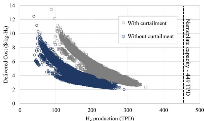
**Fig. 4 | Daily hydrogen production in metric tonnes per day (TPD) and resulting delivered cost of hydrogen to end user with and without curtailment.** Storage is sized to capture all curtailment, allowing a facility to produce hydrogen at an average daily capacity closer to the electrolyzer facility nameplate capacity.
