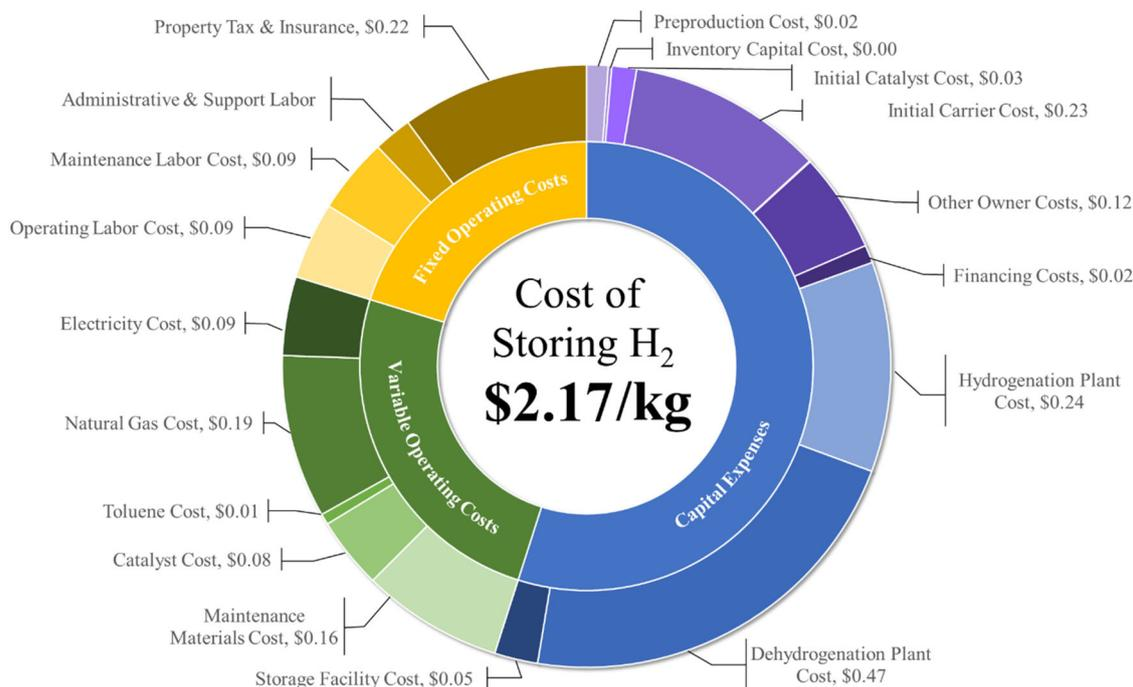
**Fig. 2 | Cost breakdown of methylcyclohexane carrier storage system at exemplary Texas site.** Breakdown of levelized cost of storage in a case where the storage facility is serving a 200 tonnes per day end user. Hydrogen storage size is 3156 tonnes.
