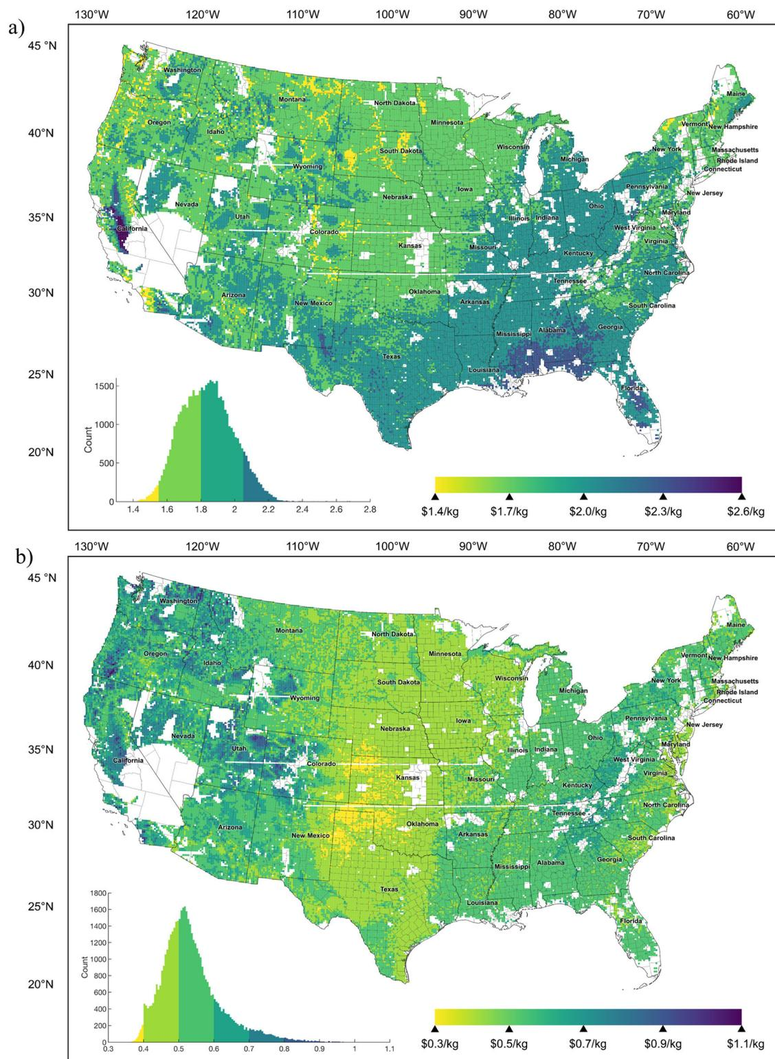
**Fig. 5 | Geographic distribution of carrier storage cost in the contiguous United States<sup>38</sup>. a** Levelized cost of storage (LCOS) for least-cost wind- and solar-based H<sub>2</sub> production sites. **b** Additional cost to end user (ACEU) that would increase the cost of produced H<sub>2</sub> depending on the quantity of H<sub>2</sub> stored.
