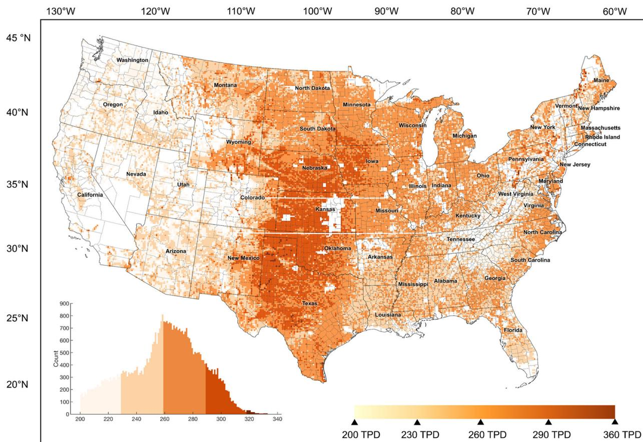
**Fig. 6 | Locations capable of serving industrial end users with 200 metric tonnes per day (TPD) or higher H<sub>2</sub> consumption in the contiguous United States<sup>38</sup>.** Locations included with a dehydrogenation capacity greater than 200 TPD.
