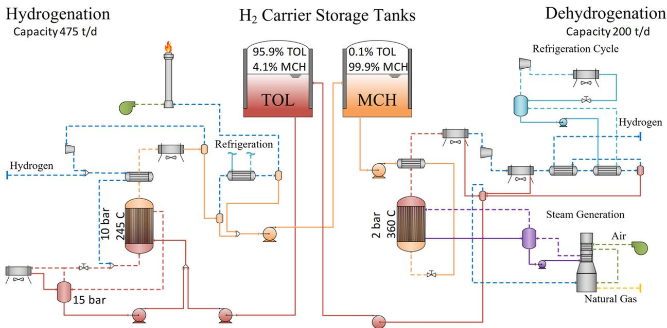
**Fig. 8 | Process flow diagram of the TOL/MCH hydrogen storage facility.** Process used to generate the Aspen Plus model. Analysis assumes H<sub>2</sub> storage is co-located with the H<sub>2</sub> from PEM electrolysis and an end use application.
