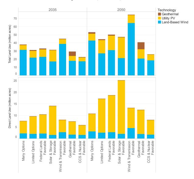
Figure 24. Total (top) and direct (bottom) land use from UPV, wind, and geothermal in 2035 (left) and 2050 (right)
