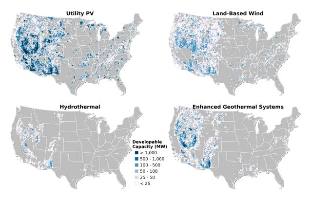
Figure 10. Developable capacity in MW on federal land for each (11.5 km) site
