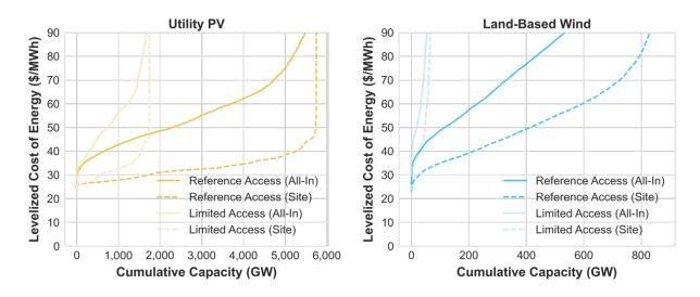
Figure 17. Federal land supply curves for UPV and wind using 2035 technology costs
