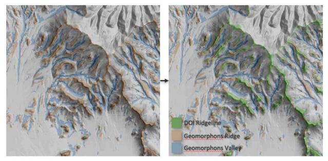
Figure B-3. Maps showing ridges and valleys derived via Geomorphons algorithm (left) and the portions of ridges meet the DOI criteria for ridgelines (right)
