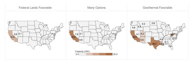
Figure 22. Geothermal installed capacity by 2035 under select scenarios
