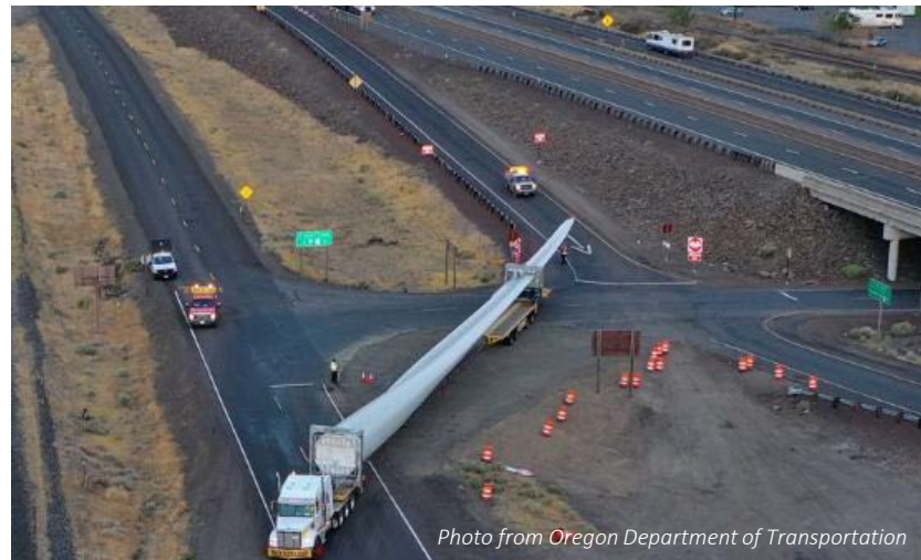
Bridge height (as low as 14 ft [4.3 m]) and limited crane capacity suppressed land-based wind turbine upscaling.
