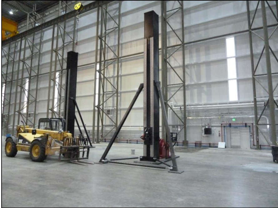
Figure 7 – Side pull towers at WTTC (12 May 2011)
