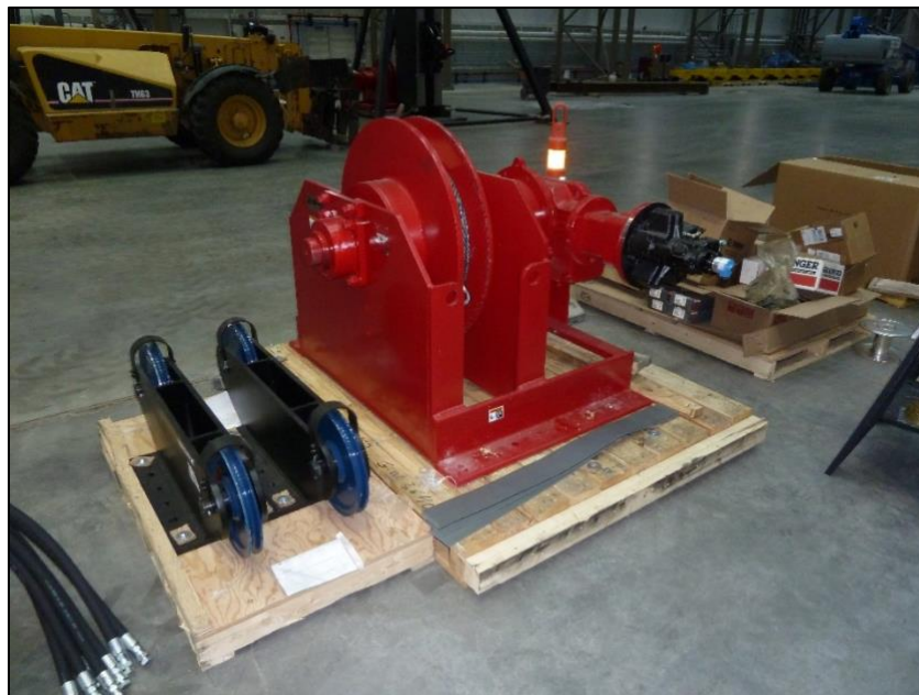
Figure 10 - Hydraulic winch and pulley systems
