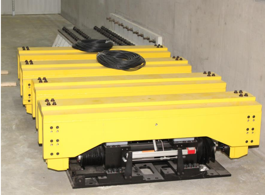
Figure 11 - UREX units including hydraulic actuators
