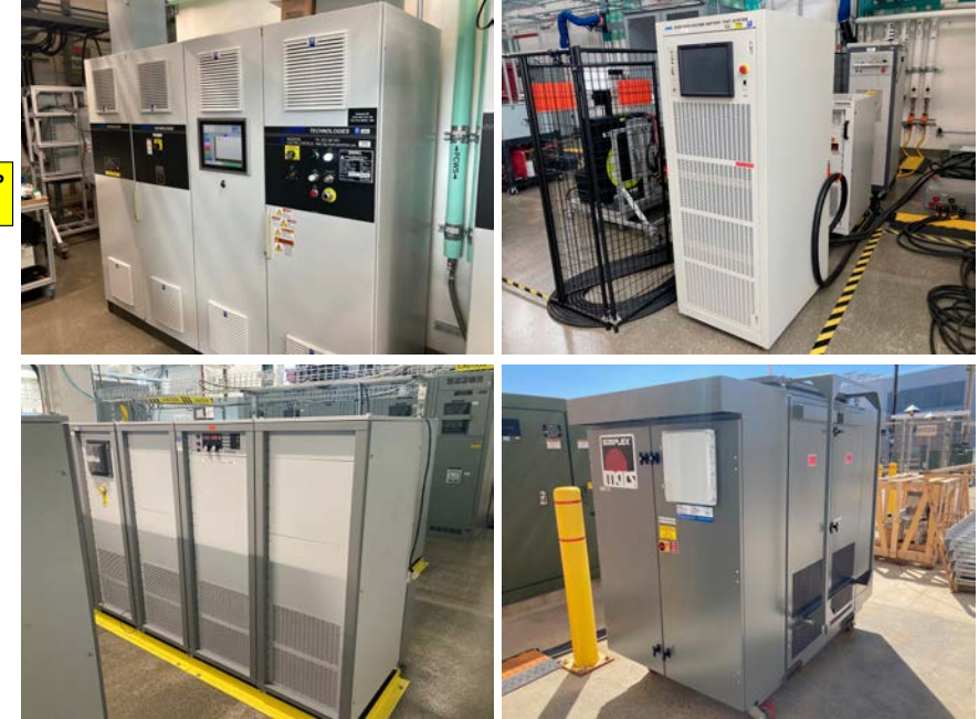
Clockwise from top left: Anderson AC2660P (GTI); NHR 9300 (EV/ EVSE Emulation); Simplex Mars (Building Load); Magna Power MTA1000-250 (PV Emulation)
