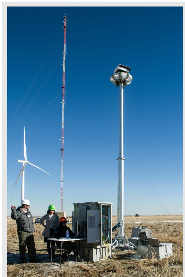
Identiflight, a camera-based mitigation technology used to reduce eagle collisions with wind turbines, is one of over 100 technologies included in the Technologies Tool. Photo by Dennis Schroeder, NREL
