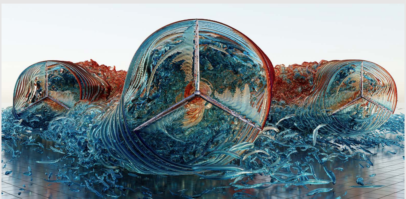
Researchers developed an ExaWind simulation of four NREL 5-MW ind turbines in a turbulent atmospheric flow, illustrated here. Graphic by Nicholas Brunhart-Lupo, NREL
