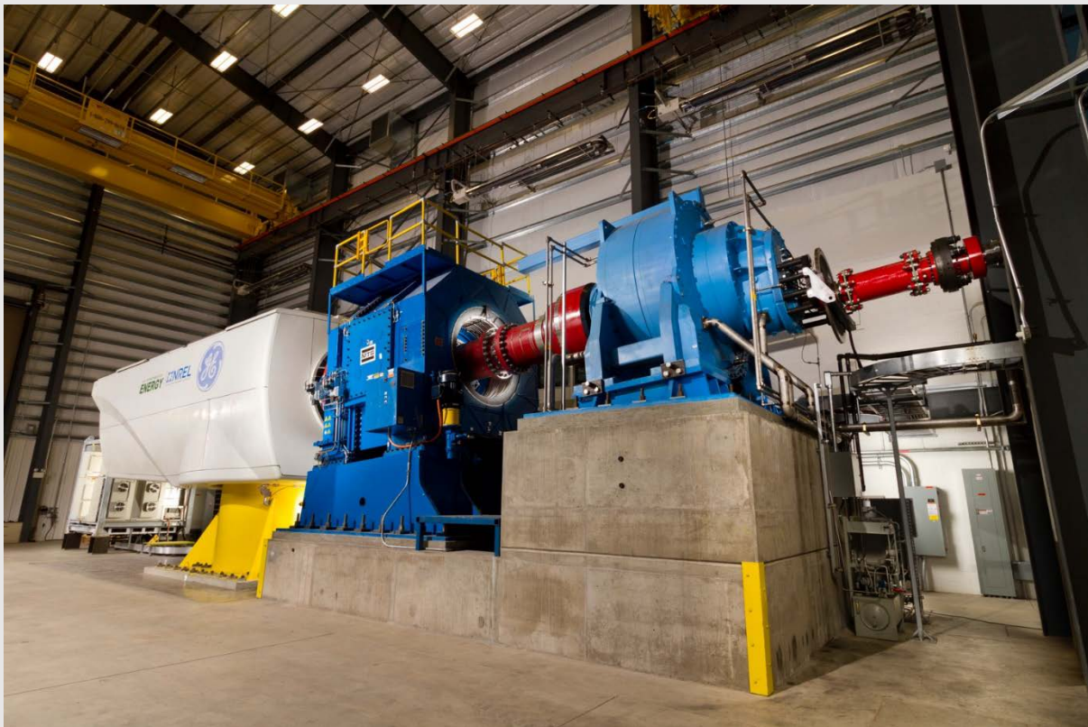
Researchers subjected GE's 2.5-MW wind turbine drivetrain, shown here attached to NREL's 5-MW dynamometer, to grid faults to validate its stability in grid-forming mode. Composite photo by Pat Corkery, Mark McDade, and Dennis Schroeder, NREL
