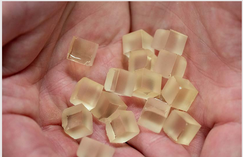
An NREL scientist holds small cubes of a new, plant-based resin for building recyclable wind turbine blades. Photo by Werner Slocum, NREL
