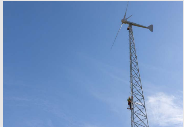
NREL's Distributed Wind Certification Best Practices Guideline offers comprehensive information and resources to help manufacturers of distributed wind energy technologies, like the Bergey Excel 15 wind turbine shown here, achieve certification so they can enter domestic and international markets. Photo by Joe Del Nero, NREL
