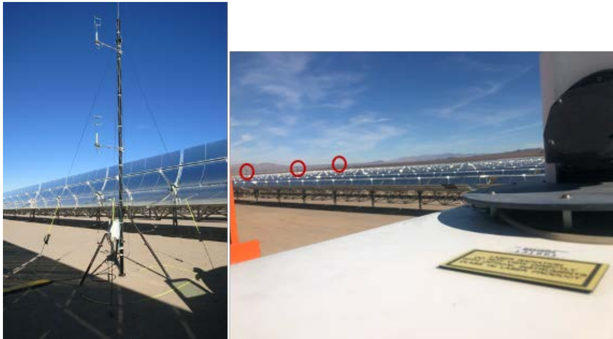
Figure 1: An 15-m tall inflow met tower (left), and locations of three 8-m tall met towers are shown with red circles in the right figure.
