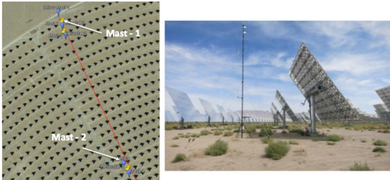
Figure 17: Met tower upwind of the heliostats (one near the edge of the plant and other in the interior of the plant) equipped with load instrumentation.
