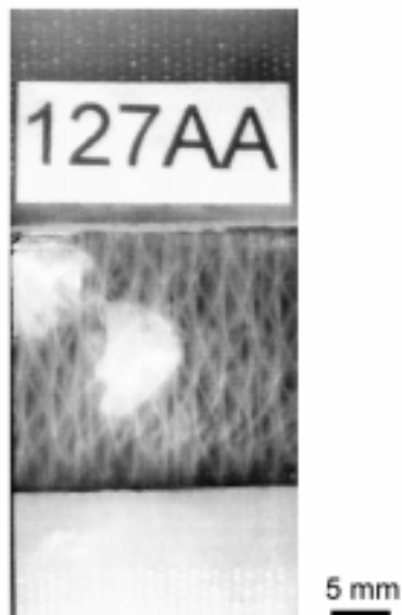
Figure 46. Delamination on a compression fatigue coupon.
