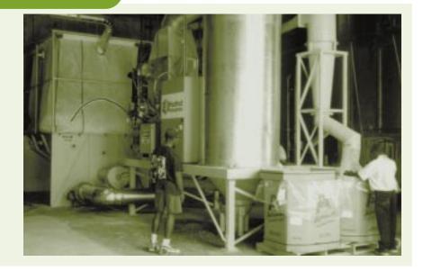
With a new thermal densification technology, many plastic foams and films, such as those used in the electronics and food packaging industries, can be successfully recovered and molded into new products.
