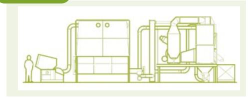
Plastic foam, ground into small pieces, is automatically fed from the hopper into the ReCyclotron via an auger and a blower. It circulates in a reaction chamber where a hot air bath floats and densifies the foam. These materials shrink, which causes them to fall out of the air stream and exit the chamber. The materials output can be conveyed into boxes or sent to a silo (not shown).
