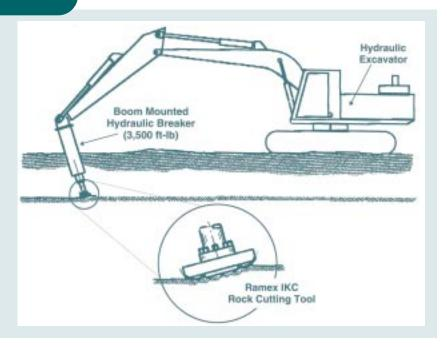
Foundation and/or trenching excavation system used to field test the Ramex IKC rock cutting tool.
