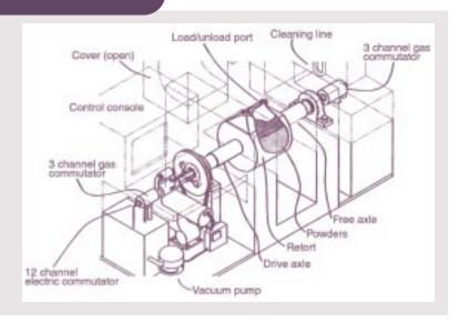
More than 500,000 tons of powdered metals are processed each year into products in the United States. By treating the metal powder before it is processed in this rotating powder treatment machine, up to 70% in energy savings and much faster production can be achieved.
