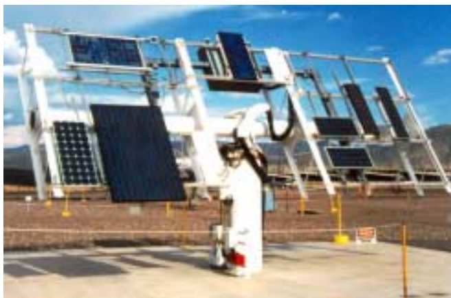
Figure 1 Sandia's computer-controlled solar tracker is used to characterize dozens of modules annually.
