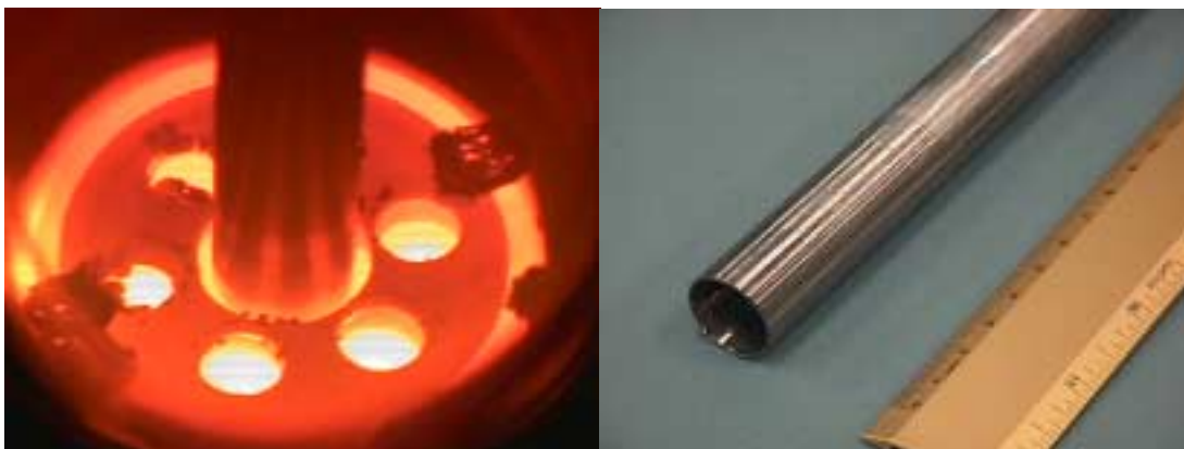
Fig. 2. The growth hot zone (left) and a resultant Si tube grown by capillary action shaping
