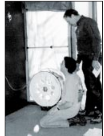
Nebraska Energy Office employee and student intern complete a blower door test in an apartment in a housing authority in Chadron, Nebraska.
