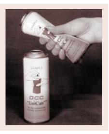
Constructing steel containers using a can's internal pressure to make the can walls rigid will save energy and reduce steel consumption and greenhouse gas emissions during manufacturing.
