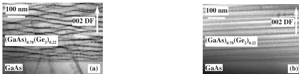
Fig. 1. 002 DF TEM micrographs of (\text{GaAs})_{0.78}(\text{Ge}_2)_{0.22} layer, grown at Spire at 675^\circ\text{C} , showing pronounced phase separation: (a) (110) cross section; (b) (\bar{1}10) cross section.
