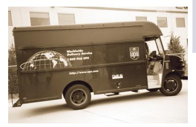
The UPS project, funded by DOE through NREL and managed by TRI, was designed to test the feasibility of using CNG in a medium-duty pick-up and delivery fleet. NREL's AFDC has logged data on the fuel use and maintenance requirements of the CNG trucks along with those of similar gasoline-powered trucks.
