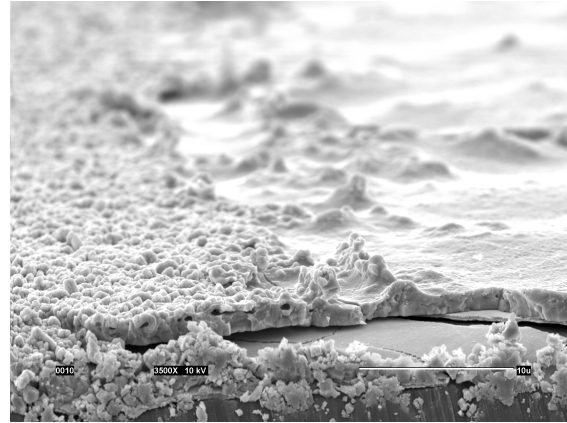
Figure 2.7. Higher magnification micrograph of front contact laser scribe showing selective removal of the ITO
