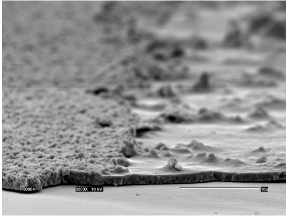
Figure 2.6. Micrograph of a front contact laser scribe on ITO/CdS/CIGS/Mo/polyimide.
