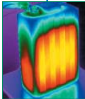
Thermal imaging of a battery used in HEVs
