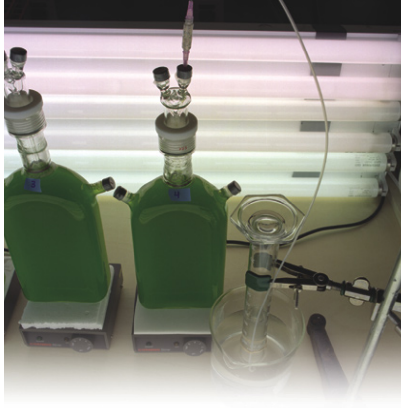
A set of bio-reactors used for photobiological hydrogen production by the green alga, Chlamydomonas Reinhardtii .
