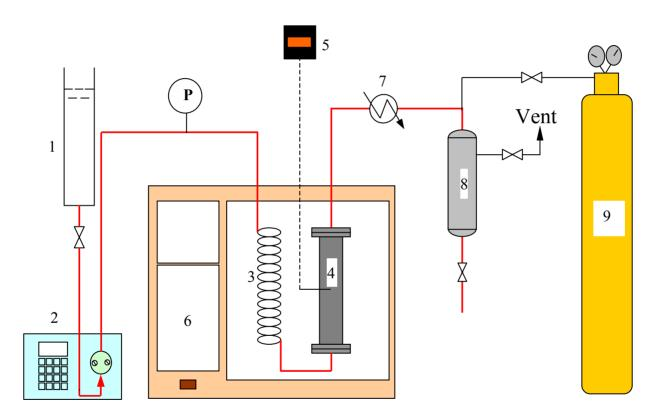
1, acid tank; 2, HPLC pump; 3, preheating coil; 4, percolation reactor; 5, thermometer; 6, GC oven; 7, heat exchanger; 8, product collecting tank; 9, N<sub>2</sub> gas.
