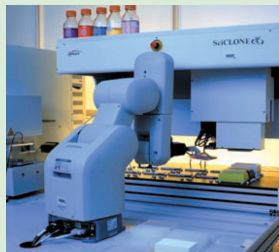
NREL scientists use a robotics deck such as this to quickly culture genetic variants of fungal genes for producing enzymes and screen them to identify the variants with the most promising characteristics.
