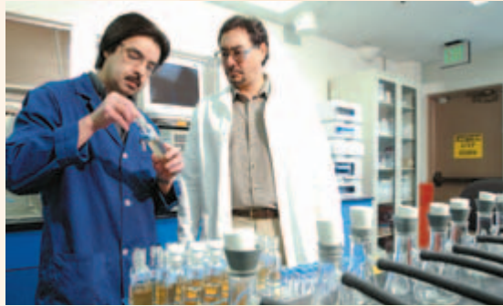
Chemists conducting compositional analysis of agricultural residue (corn stover) for carbohydrate and lignin content.
