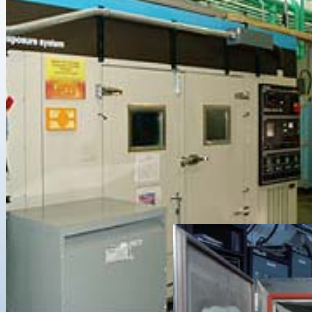
Environmental chamber for durability due to weather variations & freeze (at NREL's OTF)
