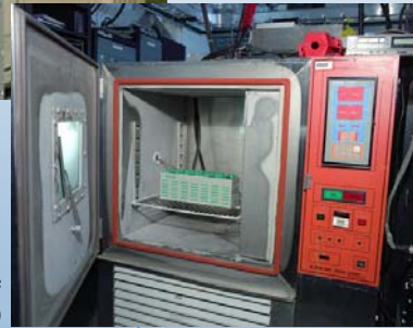
Environmental chambers for battery cold and freeze studies (at NREL's TTF)
