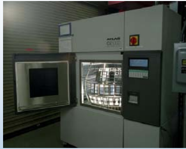
Environmental chamber for durability due to weather variations & freeze (at NREL's OTF)
