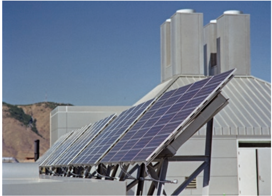
The roof of the Solar Energy Research Facility is a platform for PV panels that evaluate the performance of integrated PV systems on commercial buildings.
