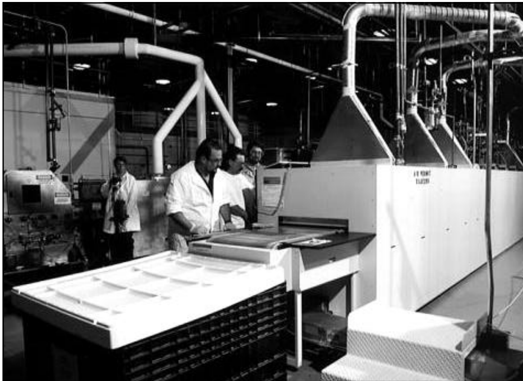
Golden Photon's facility for manufacturing cadmium telluride PV modules in Golden, Colorado
