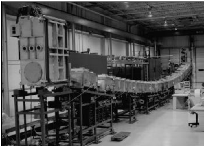
Automated production: Energy Conversion Devices can maintain very high product quality (uniformity varies less than 1%) and cell yield (greater than 99%) with its amorphous silicon thin-film production machine.
