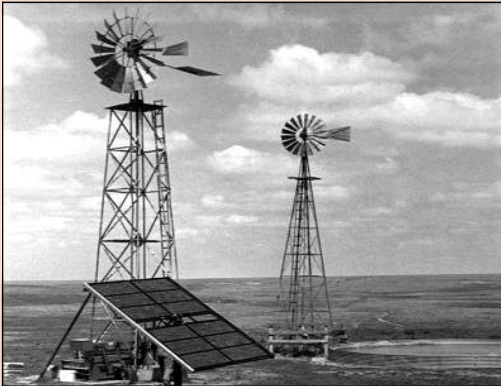
A PV-powered water-pumping station operating on the Bledsoe ranch in eastern Colorado.
