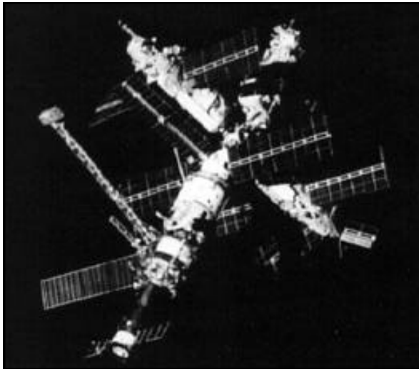
The Russian space station Mir, with PV panels extended, photographed shortly before the U.S. space shuttle Atlantis docked with it in July 1995. Photovoltaics has been used to power satellites since the late 1950s.
