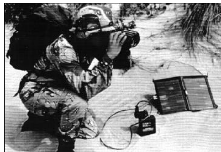
Portable photovoltaic battery chargers have been put to good use in a variety of military applications.
