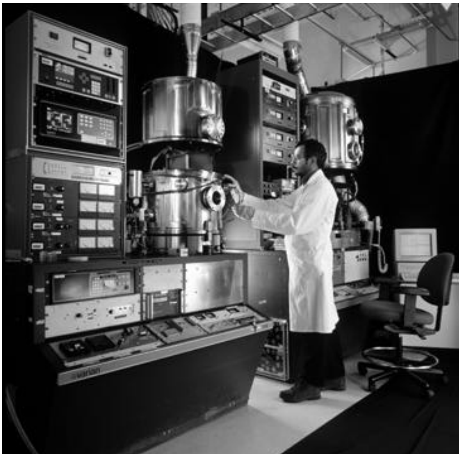
These two physical vapor deposition systems are used for making various copper indium diselenide PV cells.
