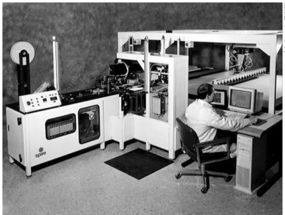
The SPI-Assembler 5000, developed under PVMaT by Spire Corporation, can reduce the cost to assemble PV modules by a factor of 5 over manual assembly methods. Two U.S. manufacturers ordered this equipment in FY 1995.
