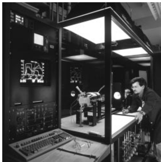
Researcher Dave Albin uses one of the close-spaced sublimation units designed and built by NREL's Cadmium Telluride Device Development team.
