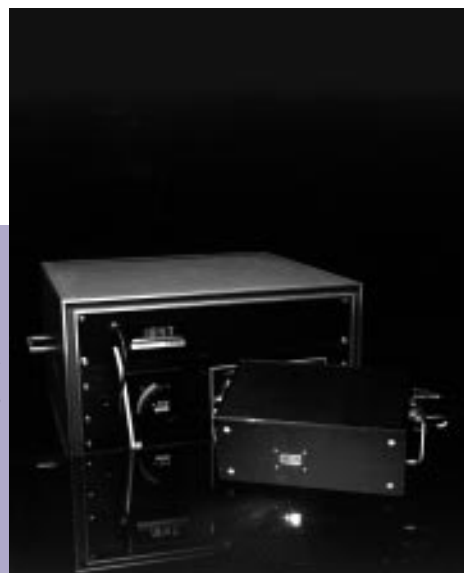
This photoluminescence-based unit can monitor the uniformity and quality of CdS/CdTe photovoltaic modules during their production.
