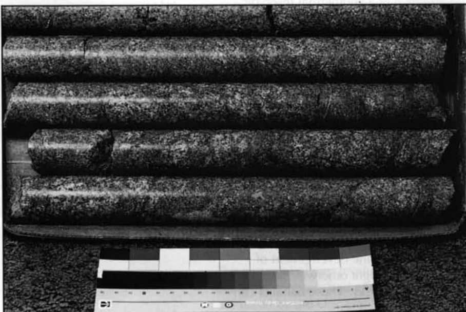
The practical application of slimhole drilling for geothermal exploration was demonstrated in FY 1993 at the Steamboat geothermal field in Nevada. Six-inch diameter core samples such as these are now being compared to the known characteristics of the field to validate the slimhole techniques.
