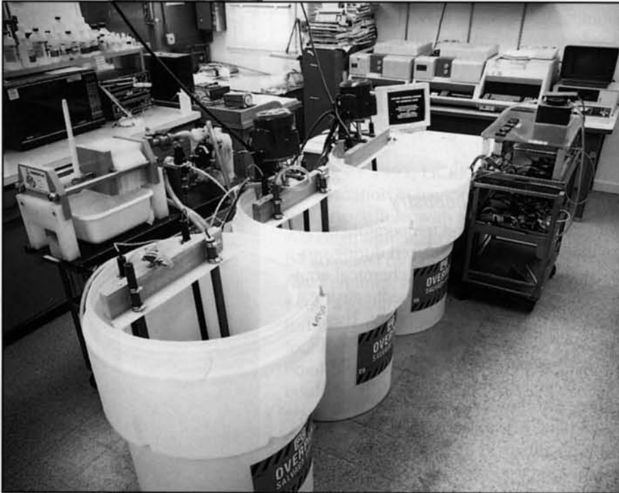
This prototype bioremediation system at Brookhaven National Laboratory was completed in FY 1993. The system will be used to optimize a process that uses bacteria to remove heavy metals from geothermal solid wastes.
