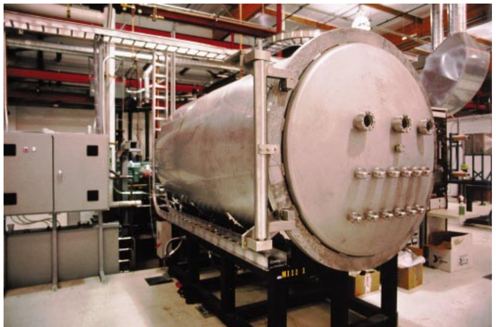
APS's deposition chamber for making 48 modules, each having a 13-ft 2 area.
