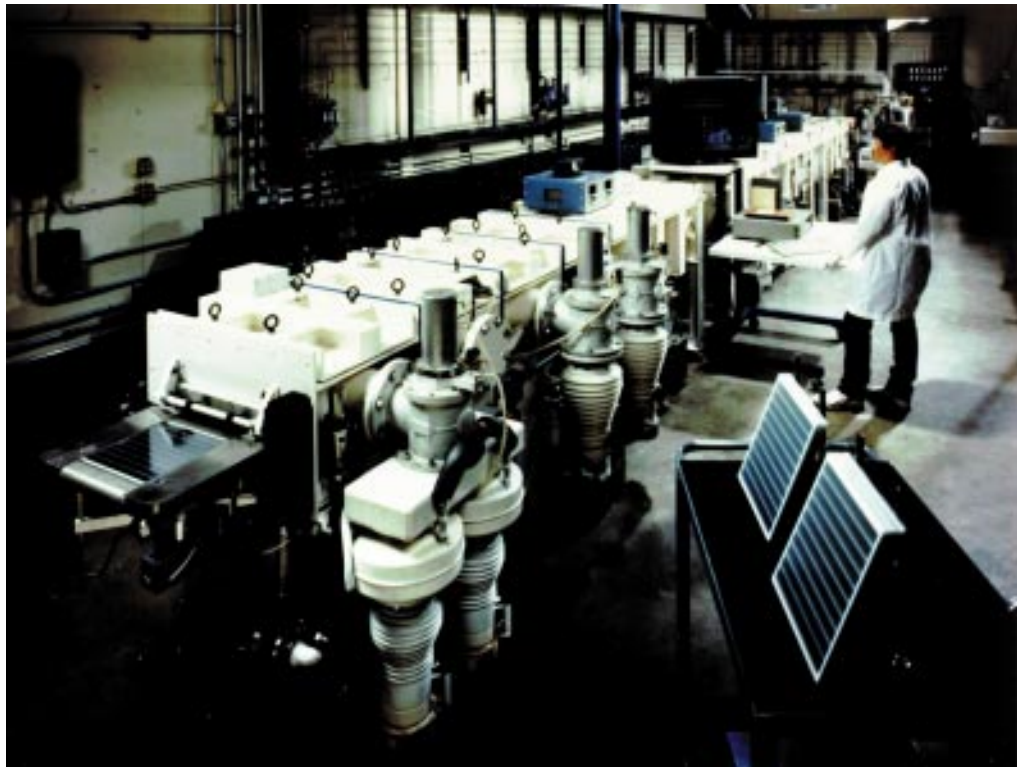
Amorphous silicon PV modules are prepared for in-line encapsulation and termination processing.
