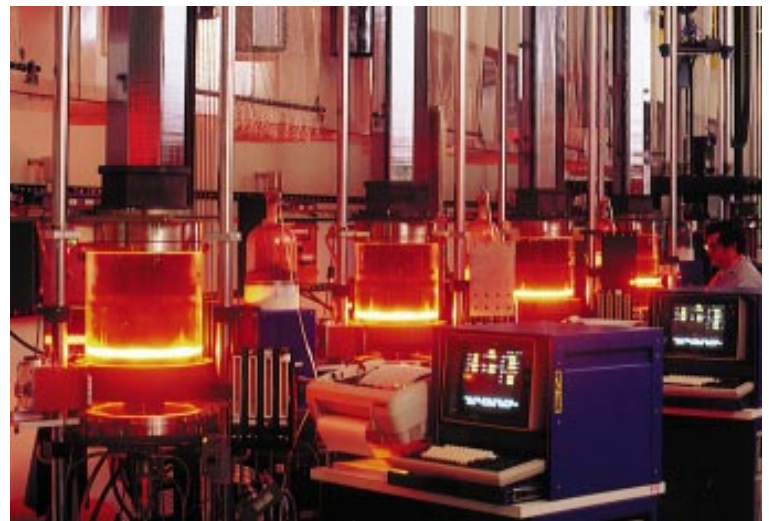
ASE Americas' production line for EFG crystal growth.
