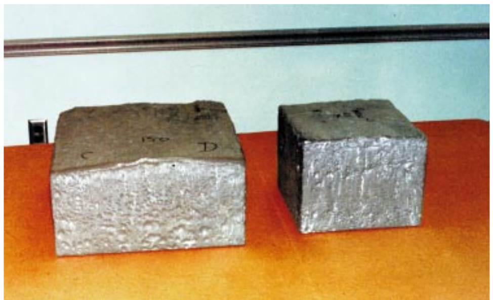
Solarex standard cast ingot versus larger size PVMaT-developed ingot.
