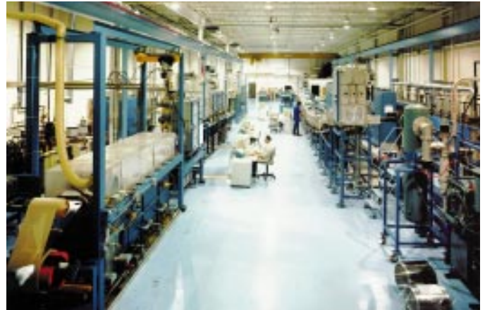
ECD's continuous roll-to-roll production line for a-Si.
